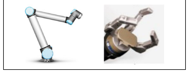
Figure 8. UR-5 robot arm and Barrett three-finger hand used in our rehabilitation robot.
