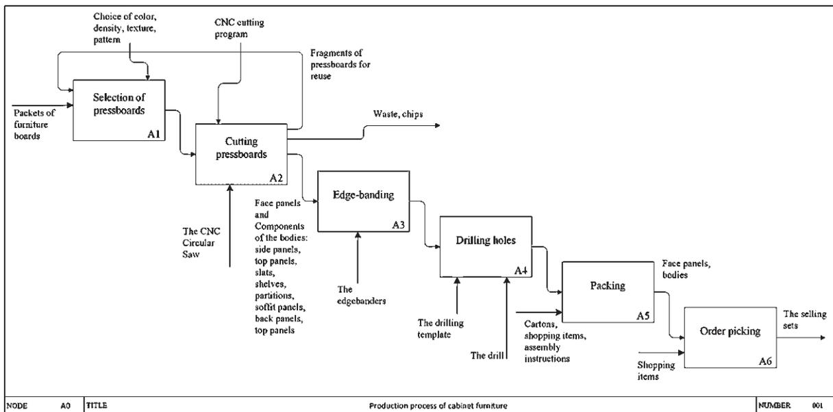
Figure 1 Diagram of cabinet furniture manufacturing process, created in IDEF0<sup>1</sup>
