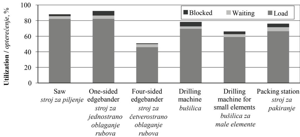
**Figure 7** Loads of machines and facilities
