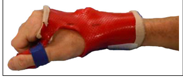
Figure 8. The figure shows the thermoformed plastic support, also known as “splint”, which has been used as a basis for the coupling between the patient's hand and the HES. HES: hand exoskeleton systems.
