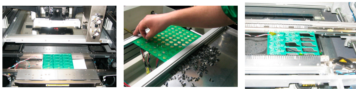
Figure 2. Solder paste printing, connector manual assembly and PCB depaneling.
