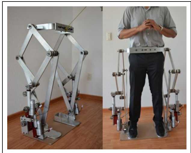
Figure 2. Prototype of the PL-based exoskeleton in construction. PL: Peaucellier–Lipkin.
