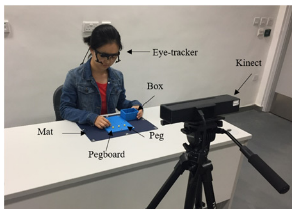
Fig. 1 Schematic diagram of the proposed system used in placing pegs task
