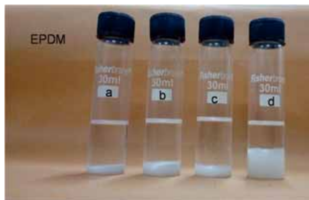
Figure 8. Swellings of (a) untreated MCC, (b) DMAc/LiCl-treated MCC, (c) untreated MCC subjected to EPDM rubber-assisted mechanical and (d) DMAc/LiCl-treated MCC subjected to mechanochemical shear.
