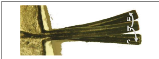
Figure 14. Drive test using different bipolar voltages.
