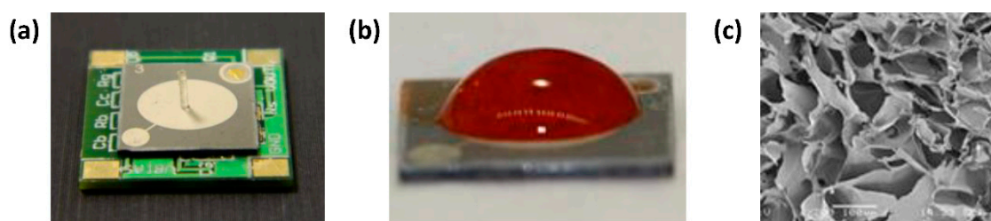
Figure 2. Canal neuromast inspired oscillatory flow sensor (a) photograph of PZT membrane with hair-like copper structure and (b) HA-MA hydrogel of Young's modulus 10 kPa. (hydrogel is coloured with rhodamine dye) (c) SEM image of the cross-section of HA-MA hydrogel cupula.
