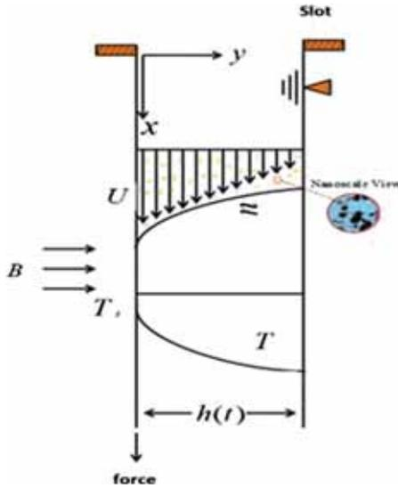
Figure 1. Geometry of the flow problem.
