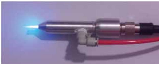
**Figure 2.** Photograph of the argon RF plasma jet in the operational conditions.
