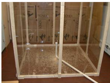
Figure 3.2. Chamber construction with Plexiglas sides, front access door, and particulate introduction pipe.
