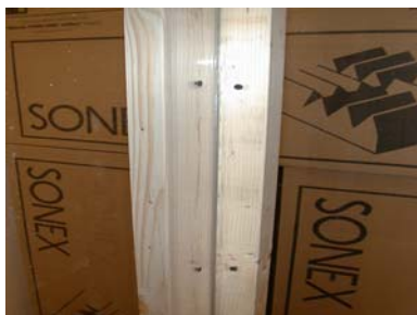
Figure 3.3. Corner of experimental chamber with fastening screws and silicone adhesion corner seal.
