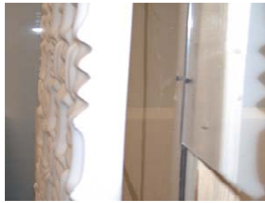
Figure 3.12. Space between the SONEX panels and the chamber wall during particulate weighing.
