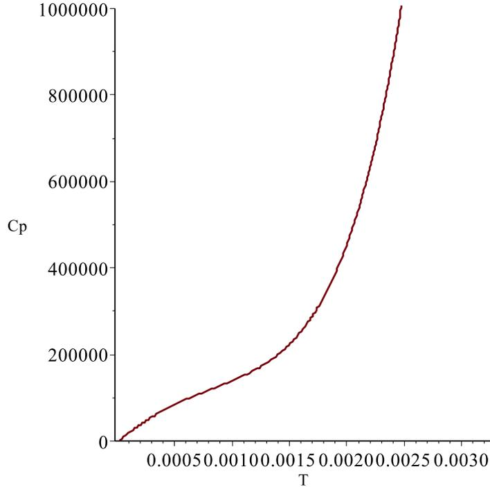
Figure 5.4: **Specific Heat.** This curve represents  $C_P$ , the specific heat of the system, as a function of the temperature. It is plotted for  $P = -0.0001$  and  $\Phi_+ = 0.1$  .
