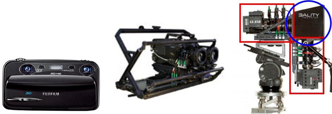
(a) Fuji FinePix REAL 3D W3: two lenses, two capture surfaces, fixed interaxial. (b) 3ality Technica TS-4: side-by-side rig, two cameras, adjustable interaxial. (c) 3ality Technica TS-5: beamsplitter rig, two perpendicular cameras, adjustable interaxial.
