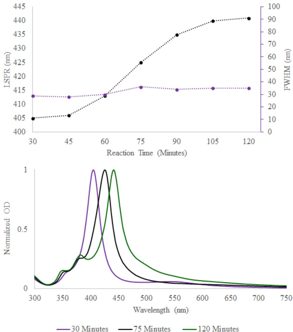
*Figure 9. Evolution of LSPR and FWHM throughout the synthesis of octahedra AgNPs (top). Normalized OD spectra of aliquots obtained from the synthesis of octahedra AgNPs after 30, 75 and 120 minutes into the synthesis.*
