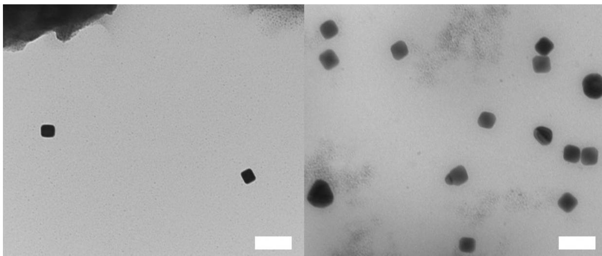
*Figure 6. TEM images of cubes (left) and octahedra AgNPs (right) after 90 minutes of synthesis. Scalebar represents 100 nm.*
