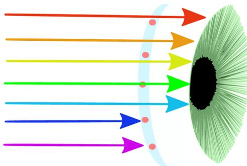
*Figure 1. Illustration of AgNP (pink spheres) integrated lenses filtering out harmful high-energy wavelengths and allowing transmission of lower energy wavelengths.*
