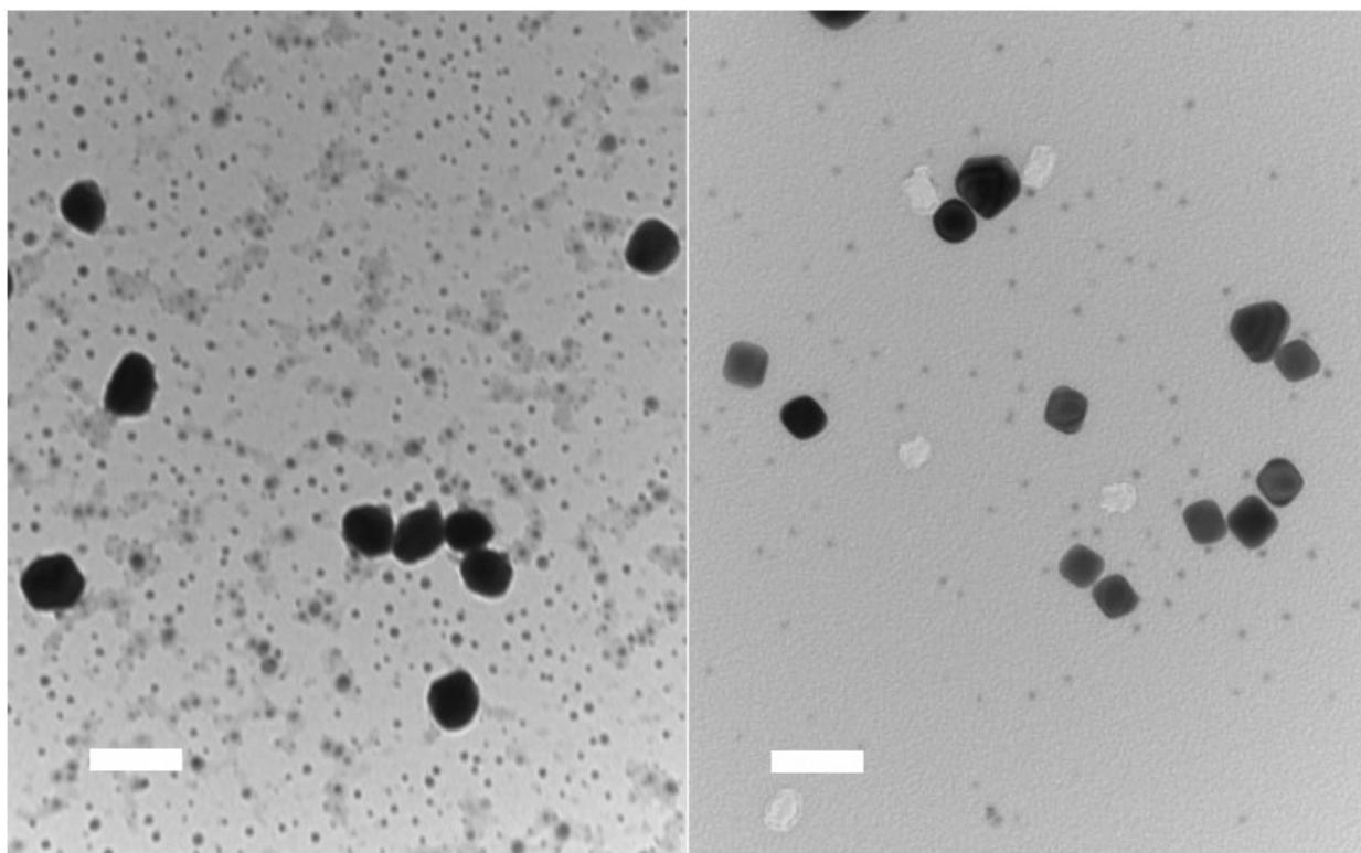
*Figure 12. TEM images of commercial AgNPs (left) and octahedra AgNPs (right) synthesized using the optimized conditions of the polyol method. Scalebars represent 100 nm.*
