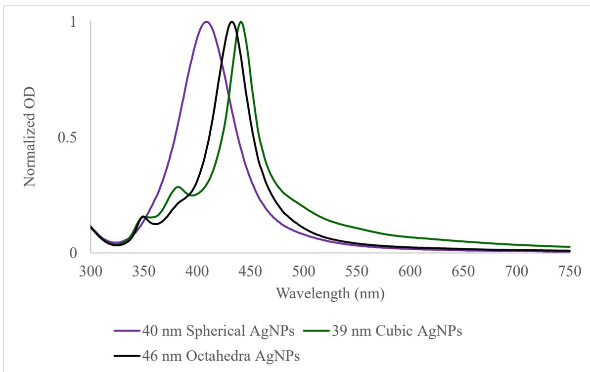
*Figure 10. Normalized OD spectras of 40 nm commercial spherical AgNPs, cubic AgNPs and octahedra AgNPs.*
