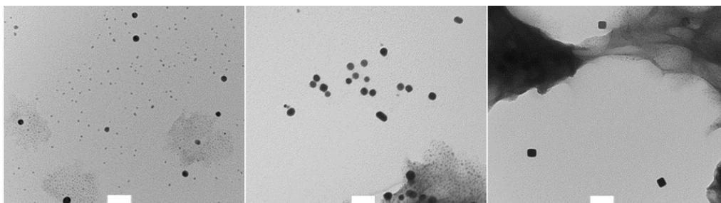
*Figure 4. TEM images of aliquots obtained during the synthesis of cubic AgNPs after 30 (left), 45 (middle) and 90 (right) minutes. Scale bar represents 100 nm.*
