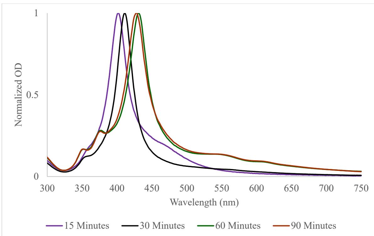
*Figure 7. Normalized OD spectra of aliquots obtained at different timepoints during the synthesis of octahedra AgNPs (60 ul NaHS).*
