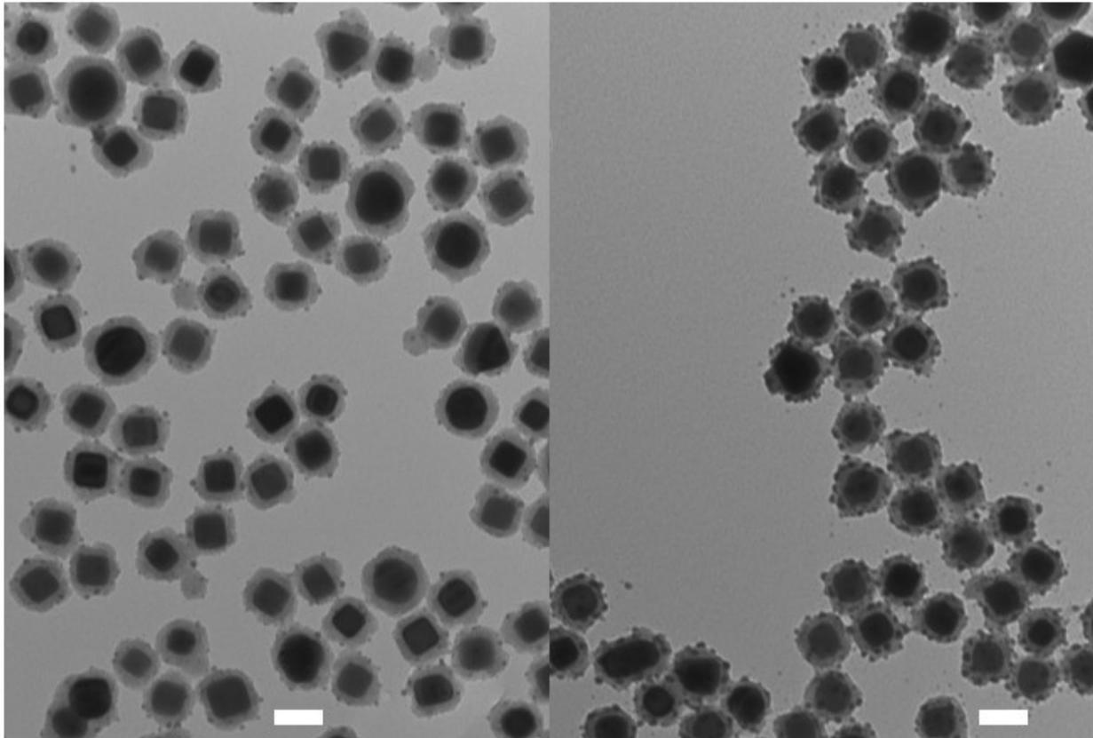
*Figure 14. TEM images of silica-coated cubic AgNPs stored in the fridge (left) and after 2 weeks of storage at room temperature (right). Scalebars represent 50 nm.*
