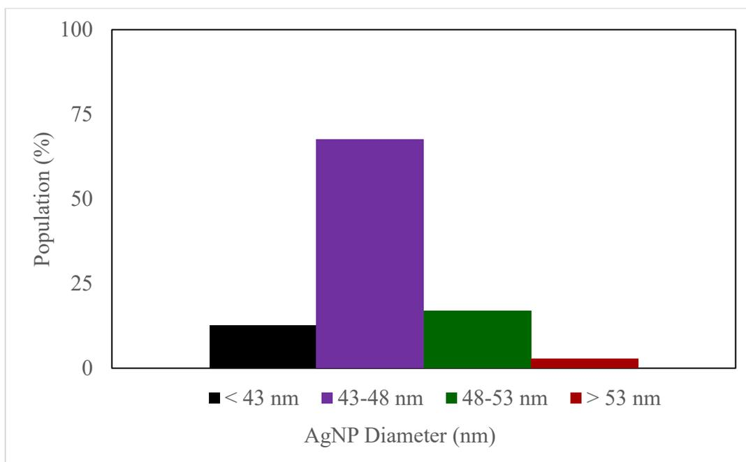
*Figure 19. Histogram showing the diameter distribution of octahedra AgNPs synthesized after 120 minutes under optimized polyol synthesis conditions.*
