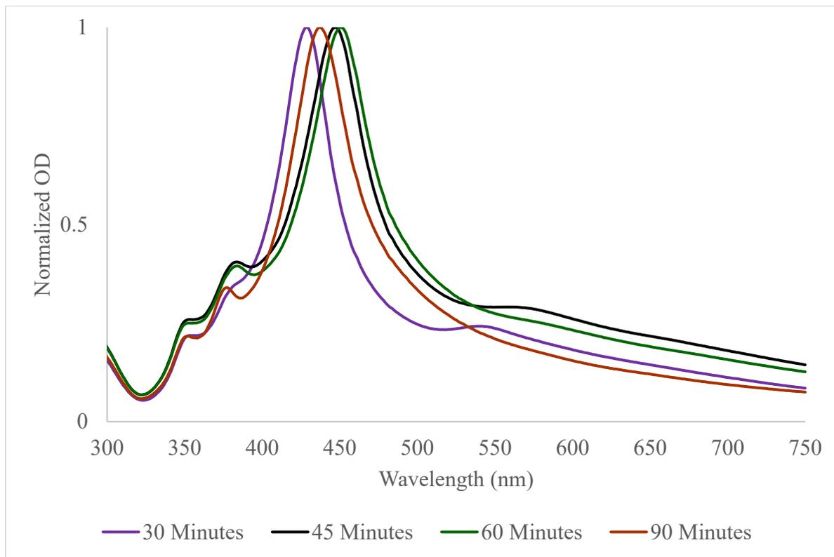
*Figure 5 Normalized OD spectra of aliquots obtained at different timepoints during the synthesis of octahedra AgNPs.*
