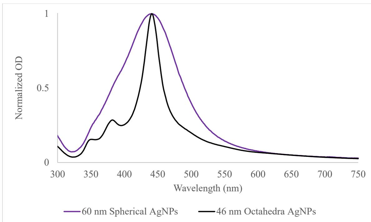
*Figure 11. Direct comparison of the normalized OD spectra of commercial spherical AgNPs and octahedra AgNPs with comparable LSPR peaks.*
