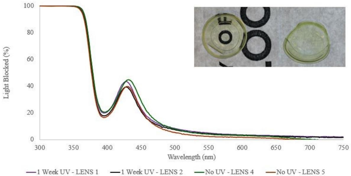
Figure 17. Light blockage profile of control NP-integrated lenses and lenses that received the equivalent of “1 week” of UV dose. The inset depicts NP-integrated lenses that received 1 week of UV exposure (left) control NP-integrated lenses (right).
