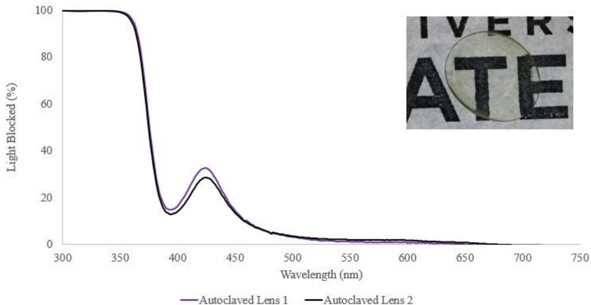
Figure 18. Light blockage spectra of autoclaved lenses. Inset depicts AgNP-integrated lens post-autoclaving.
