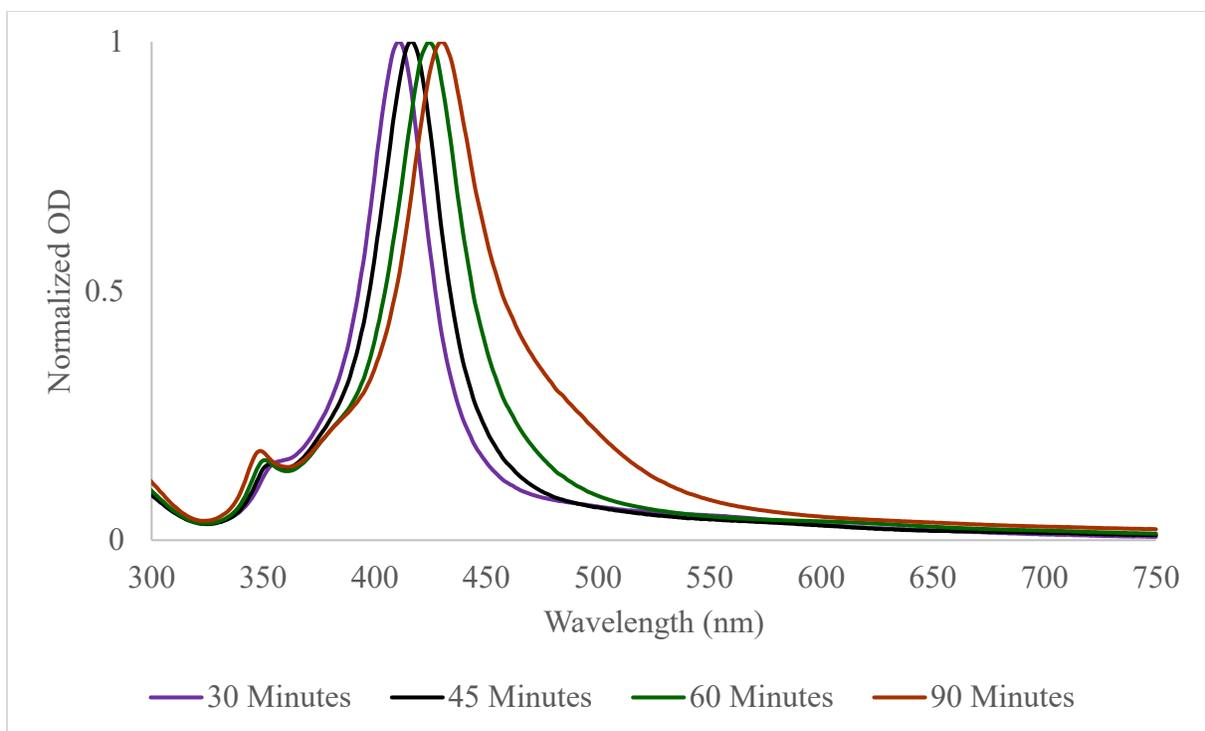
*Figure 3. Normalized OD spectra of aliquots obtained at different time points during the synthesis of cubic AgNPs.*
