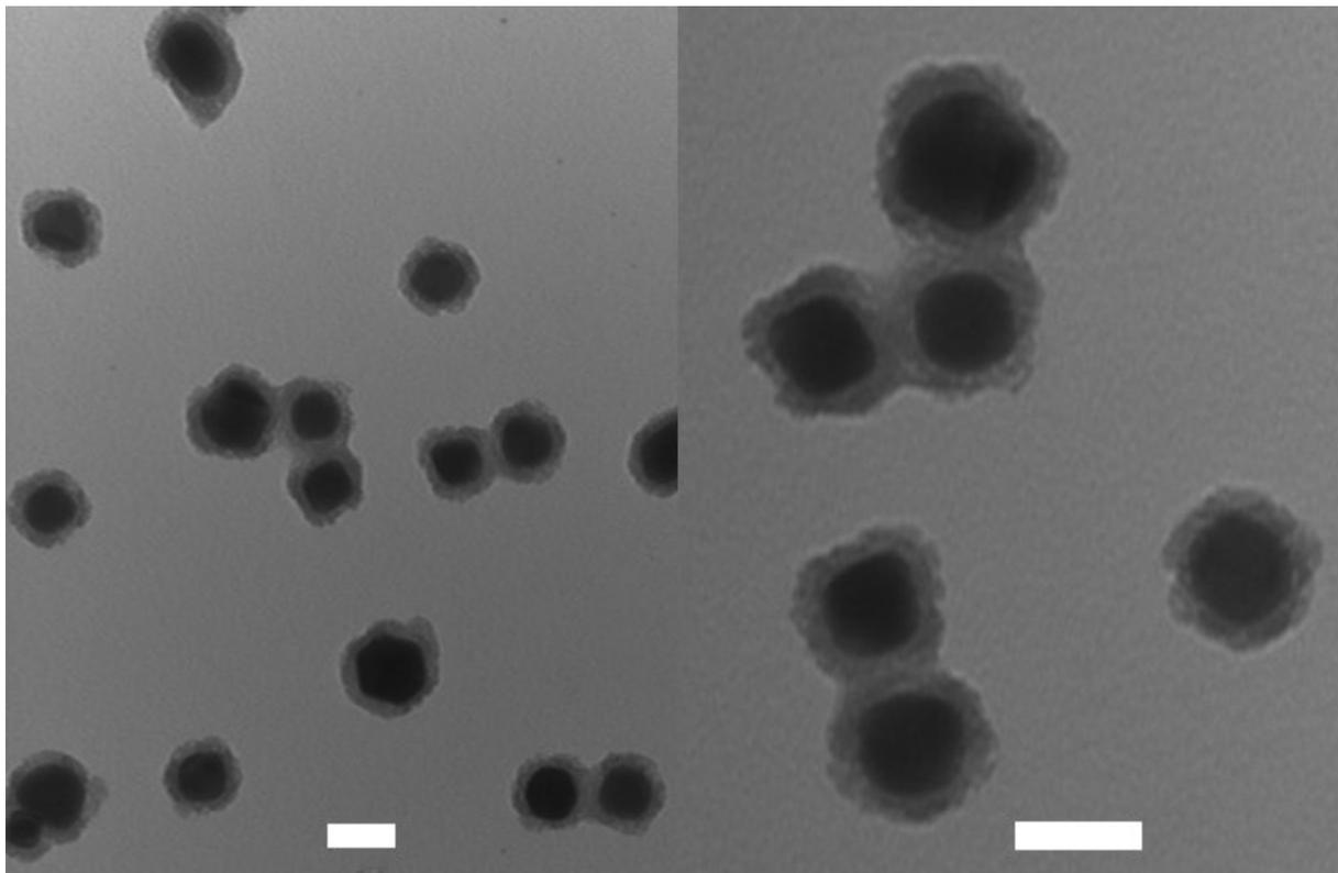
Figure 20. TEM images of octahedra NPs after silica coating (and washing). Scalebars represent 50 nm.
