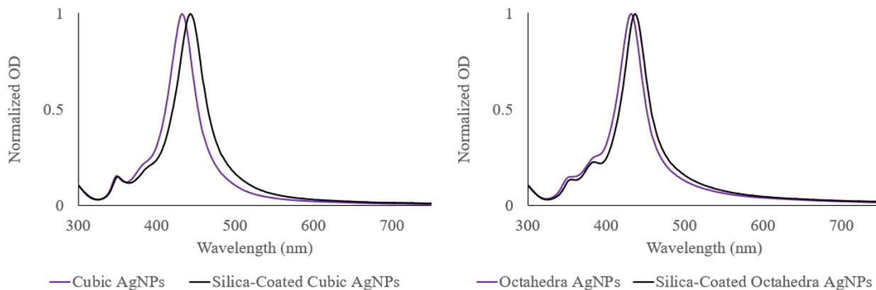
Figure 13. Normalized OD spectras of cubic AgNPs (left) and octahedra AgNPs (right) before and after silica coating.
