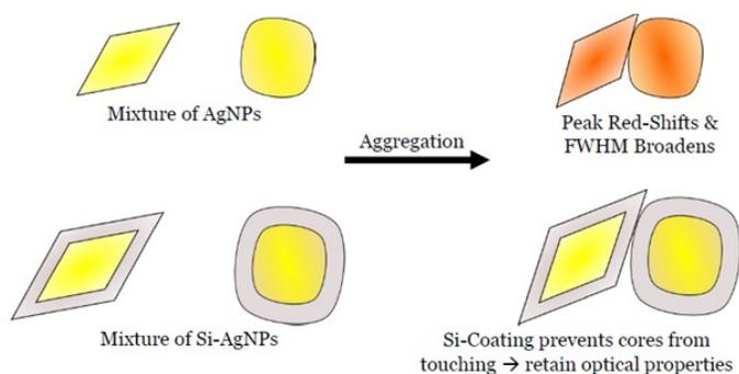
*Figure 2. Schematic illustration depicting how optical properties are preserved due to silica acting as a spacer layer between plasmonic nanoparticles in close proximity.*
