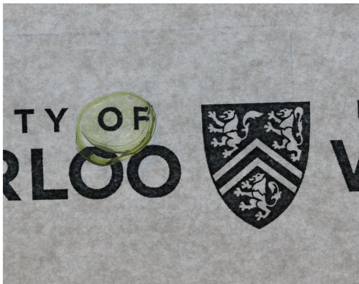
*Figure 15. NP-integrated lenses show high transparency and are devoid of visible defects.*
