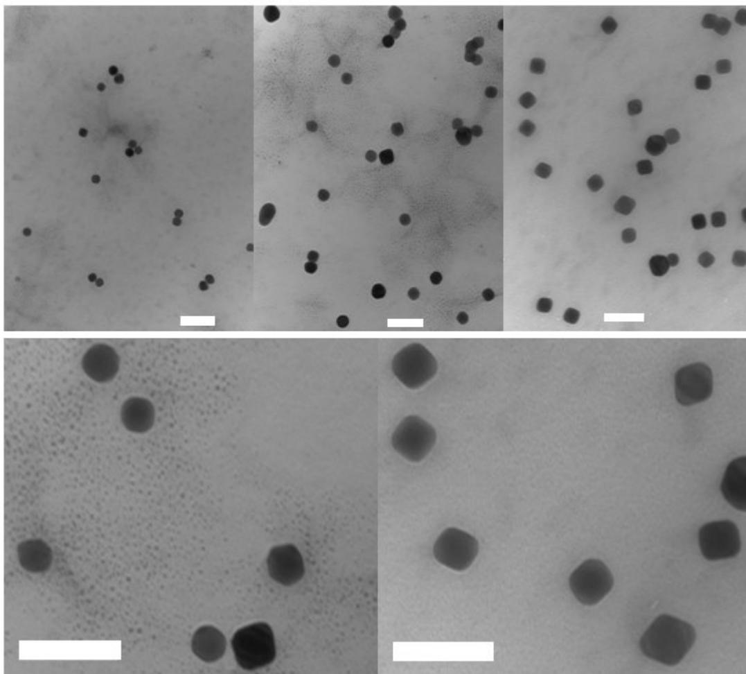
*Figure 8. AgNP growth after 15 (top and bottom left), 30 (top middle) and 90 (top and bottom right) minutes into the synthesis. Scalebars represent 100 nm.*
