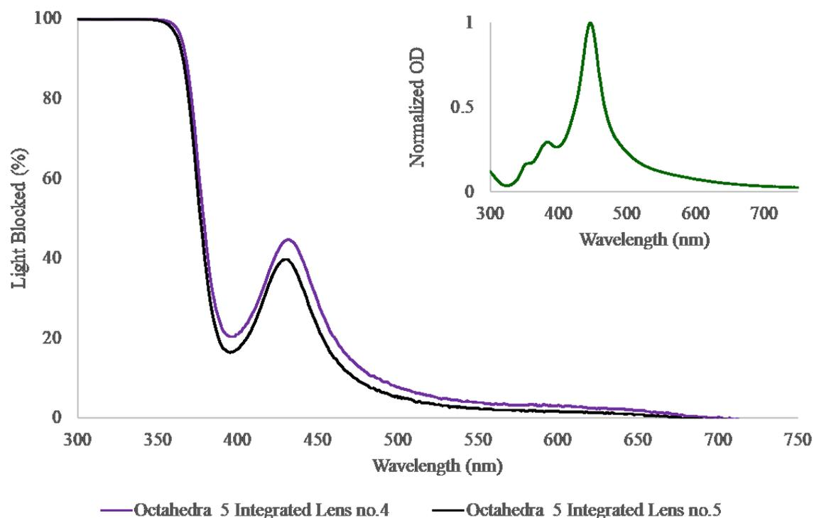
Figure 16. Light blockage spectra of lens no.4 and 5 of silica-coated octahedra AgNP-integrated etafilcon lenses. Inset is the normalized OD spectra of silica-coated octahedra AgNPs (in water) prior to integration.
