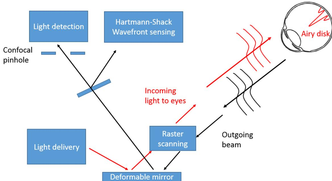
**Figure 2. 7 Schematic of Adaptive optics scanning laser ophthalmoscopy**
