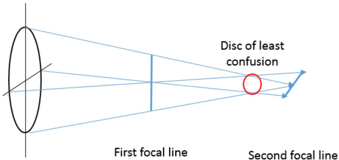
**Figure 1. 6 Schematic of astigmatism, in this case, plotted as against the rule astigmatism where the high power meridian (maximum curvature) is in a horizontal direction.**
