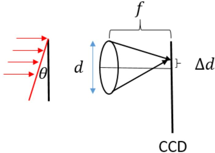
**Figure 2. 3 Schematic showing wavefront slope  $\theta$ , displacement  $\Delta d$ , focal length  $f$  and diameter of lenslet  $d$  .**
