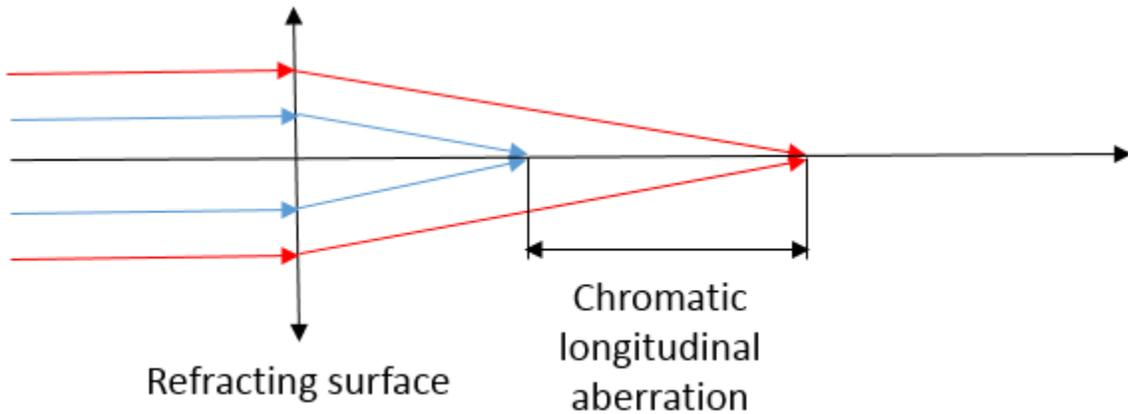
**Figure 1. 3 Schematic of longitudinal chromatic aberration**
