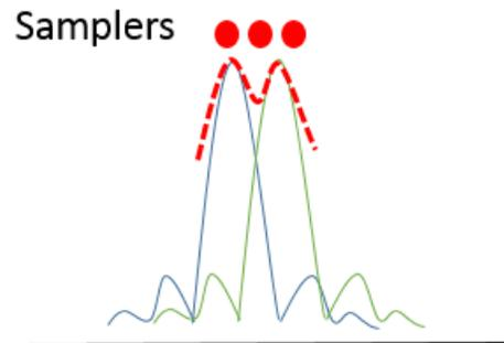
**Figure 1. 8 Rayleigh optical criterion for distinguishing two point stimuli with equal intensity: they are resolved when the zero of one PSF coincides with the peak of the other PSF. Thus the separation of the two points that can just be resolved equals the radius of the Airy disk. The red dots represent the maximum cone spacing which will still sample the two point sources given by Shannon's sampling theorem. Each of two cones sample the peak of each stimulus and a third**
