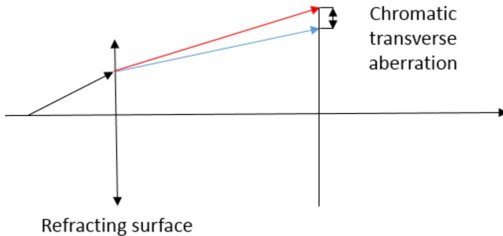
**Figure 1. 4 Schematic of transverse chromatic aberration**
