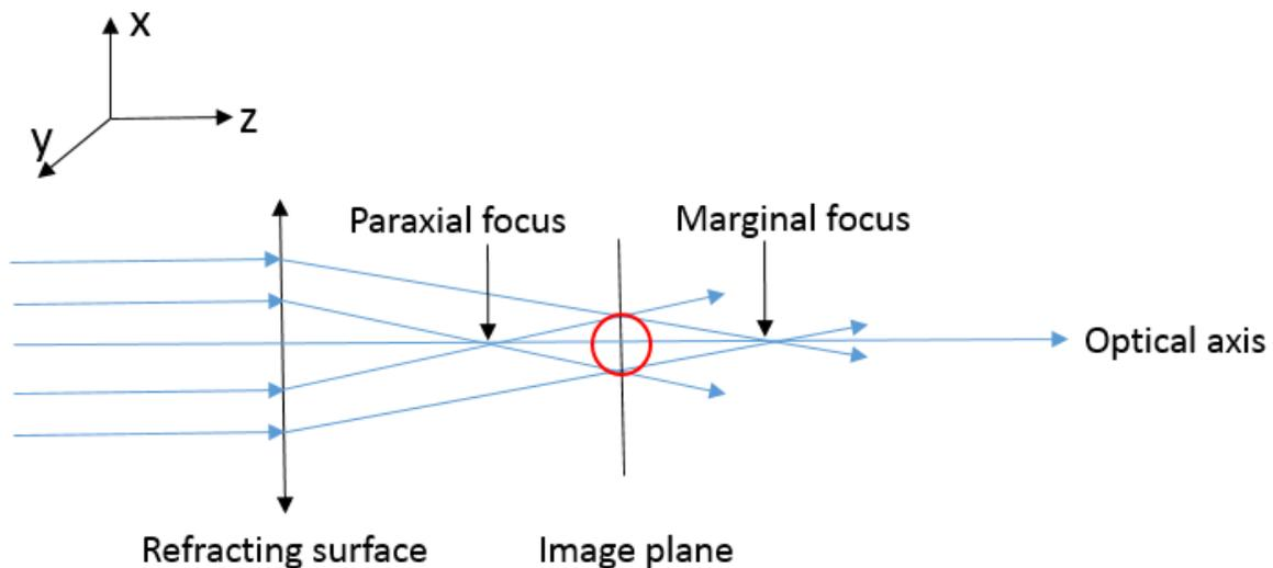
**Figure 1. 7 Schematic of spherical aberrations, in this case, the disk of least confusion sits on the image plane (retina) if only spherical aberration is present in the Zernike expansion. The spherical defocus term tells you how far the disc of least is from the retina.**
