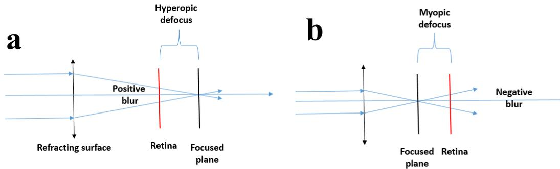
**Figure 3. 2 Schematic of the relationship between blur sign and defocus of the eye, hyperopic defocus with positive blur; myopic defocus with negative blur.**
