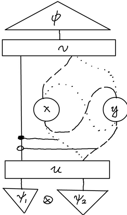
Figure 3.2: A QFT “quantum switch”. The initial state  $\psi = \psi_1 \otimes \psi_2$  factors into a qubit controlling part and the rest. When  $|\psi_1\rangle = |0\rangle$ ,  $\psi_2$  goes through  $y$  and then  $x$ . When  $|\psi_1\rangle = |1\rangle$ ,  $\psi_2$  goes through  $x$  and then  $y$ . For  $|\psi_1\rangle$  in a superposition  $|\psi_2\rangle$  goes through  $x$  and  $y$  in a quantum superposition of order.
