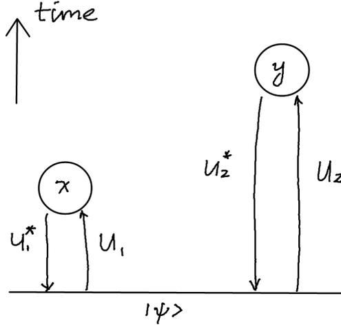
Figure 3.1: Ordinary QFT correlation function with the untilde elements. The state at a fixed reference time must be evolved by the global time evolution before being acted on by the tilde operators. Alternatively, the tilde operators must be evolved conjugatedly before acting on the state.
