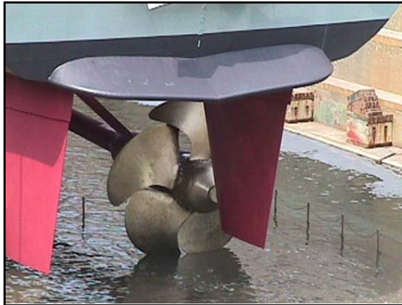
Figure 3. Stern Flap on DDG-51 Class Destroyer
