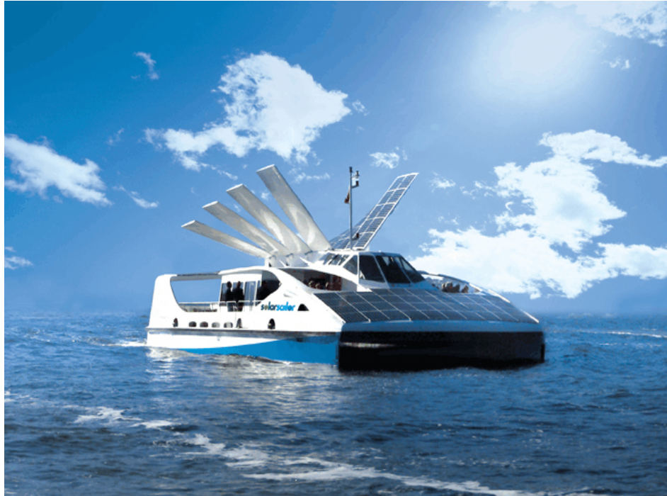
Figure 11. Solar Sailor Hybrid-Powered Ferry Boat
