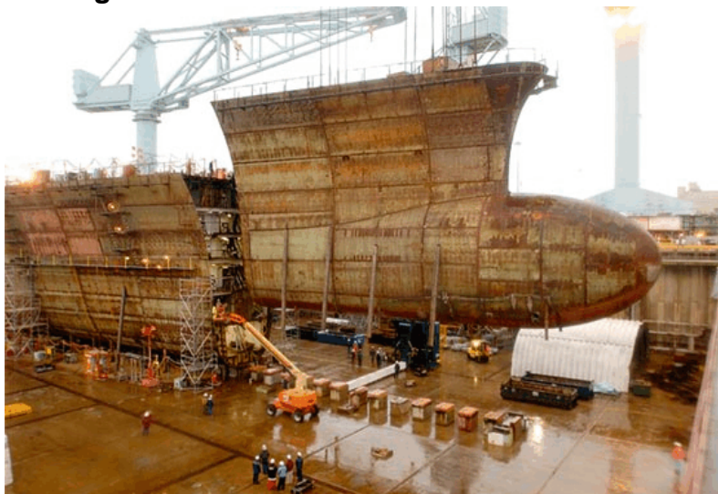
Figure 1. Bulbous Bow Section for CVN-77
