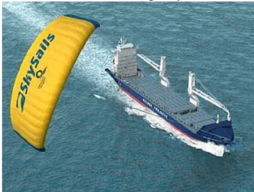
Figure 9. SkySails Concept Applied to Commercial Cargo Ship
