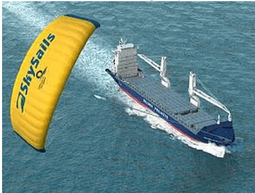
Figure 9. SkySails Concept Applied to Commercial Cargo Ship
