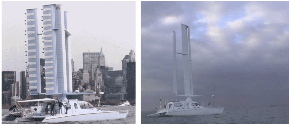
Figure 6. Pleasure Craft Equipped with Walker Wingsails
