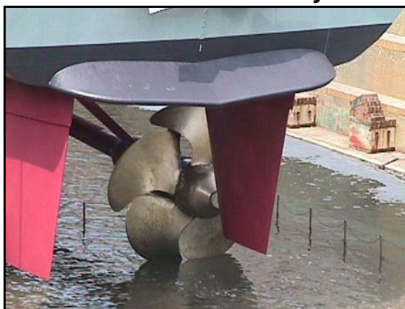
Figure 3. Stern Flap on DDG-51 Class Destroyer
