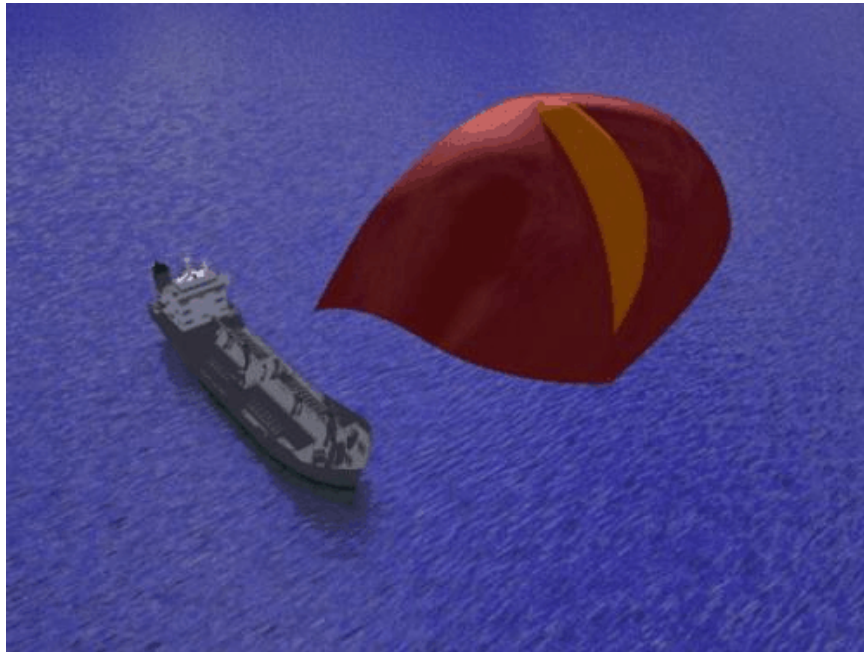
Figure 8. KiteShip Concept Applied to Commercial Cargo Ship
