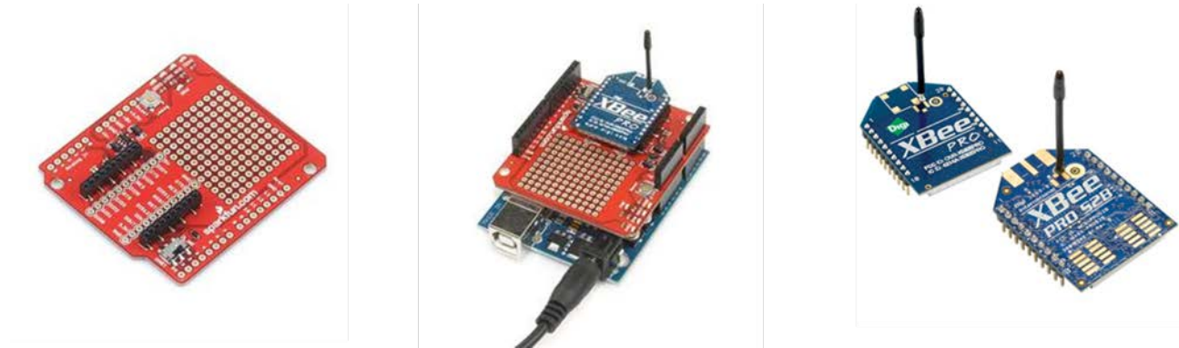
Figure 2 Arduino Xbee Shield Adaptor, Arduino Xbee Shield Assembled, Xbee with Antenna
