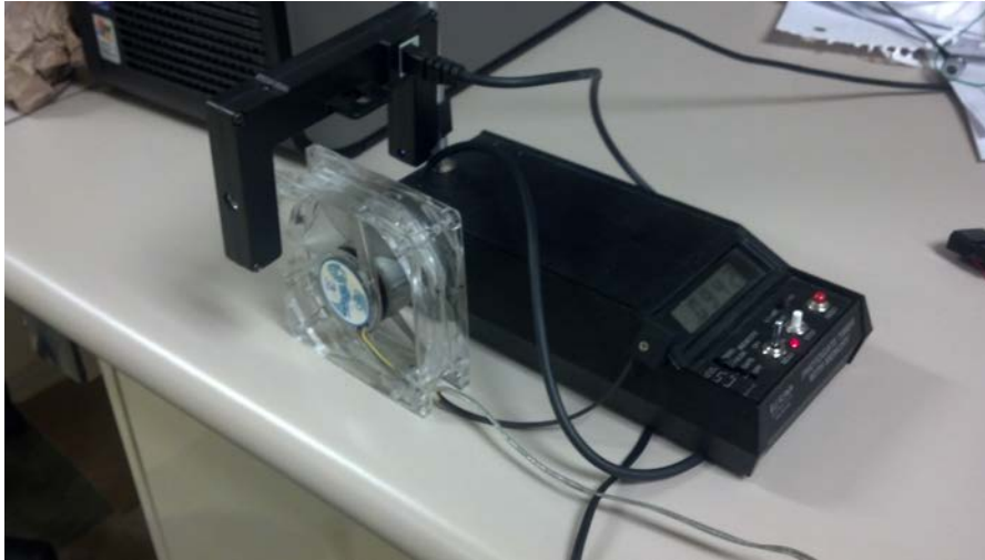
Figure 7- Photogate and fan
