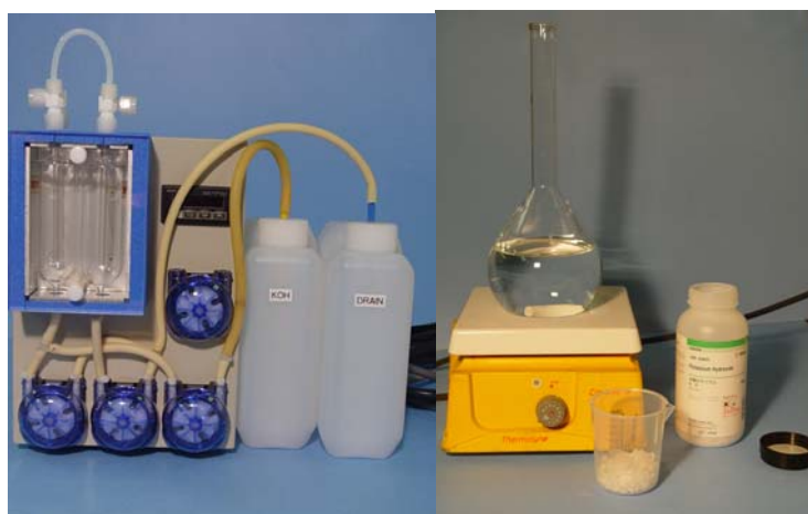
Figure 2.3.3.4 Hg CEM flue gas conditioning unit
