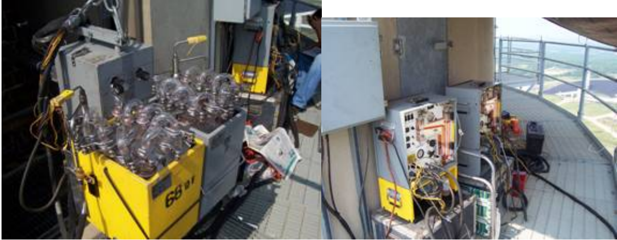
Figure 2.3.1.3 Photographs of the Ontario-Hydro rotameters and impingers at the stack
