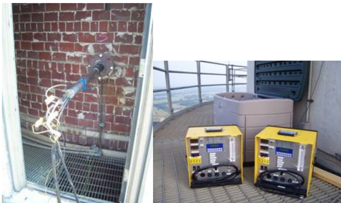
Figure 2.3.2.5 Photographs of the Method 324 equipment and penetration at the stack
