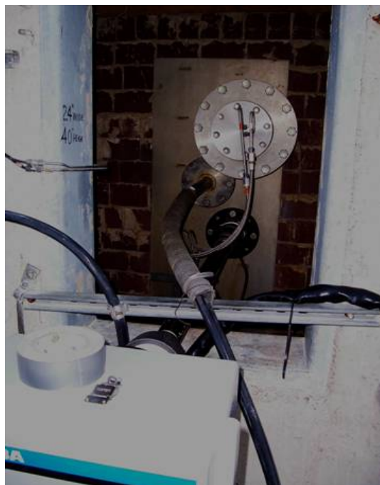
Figure 2.3.3.3 Hg-CEM system penetration into the stack
