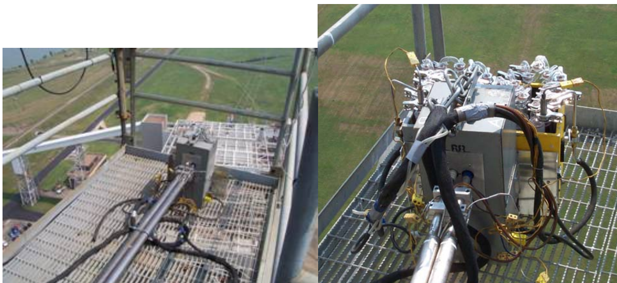
Figure 2.3.1.2 Photographs of the Ontario-Hydro probe at the stack
