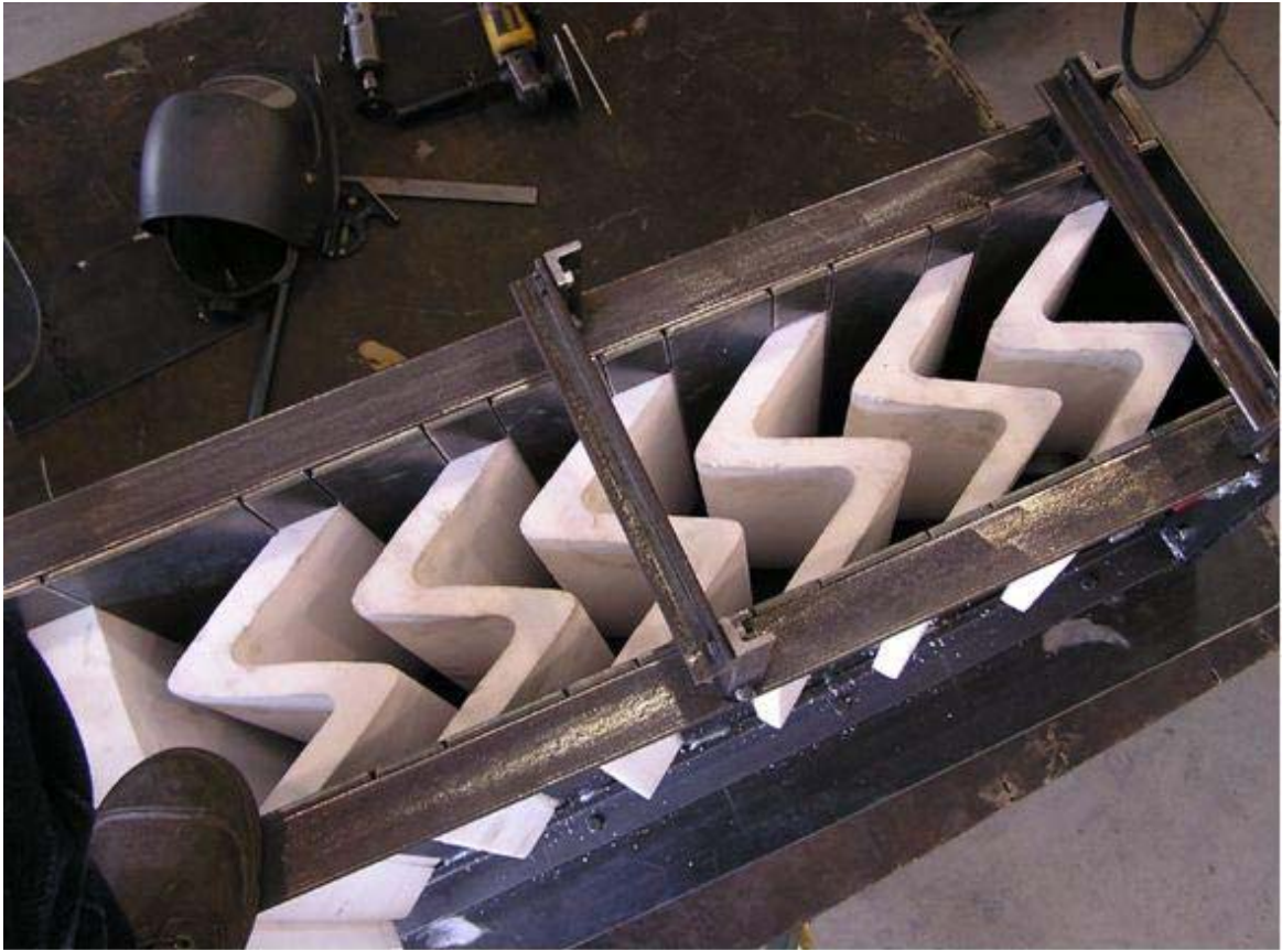
Figure 18: Photograph of the manufactured zigzag channel for insertion in the tundish.
