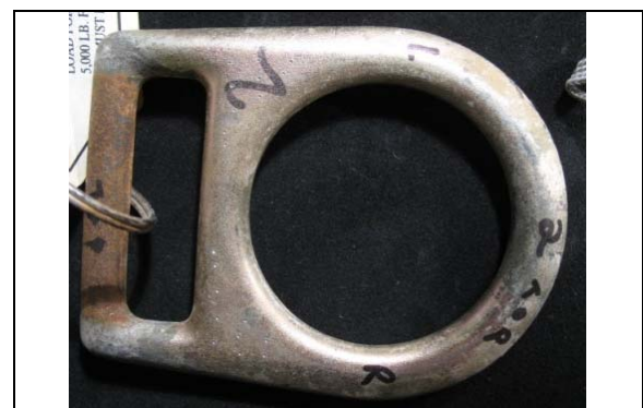
FIGURE 11 Corroded D-ring Sample 2DRC with Indents.
