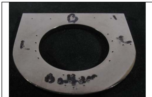
FIGURE 8 As-Received Yoke Sample NiARY1 with Indents.
