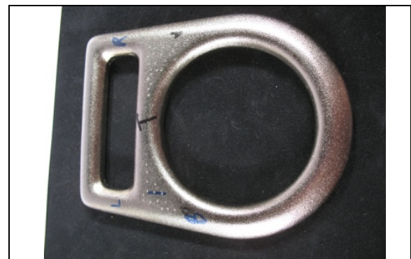
FIGURE 9 As-Received D-ring Sample NiARDR1 with Indents.
