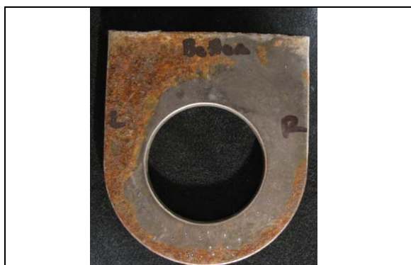
FIGURE 10 Corroded Yoke Sample 2YC with Indents.
