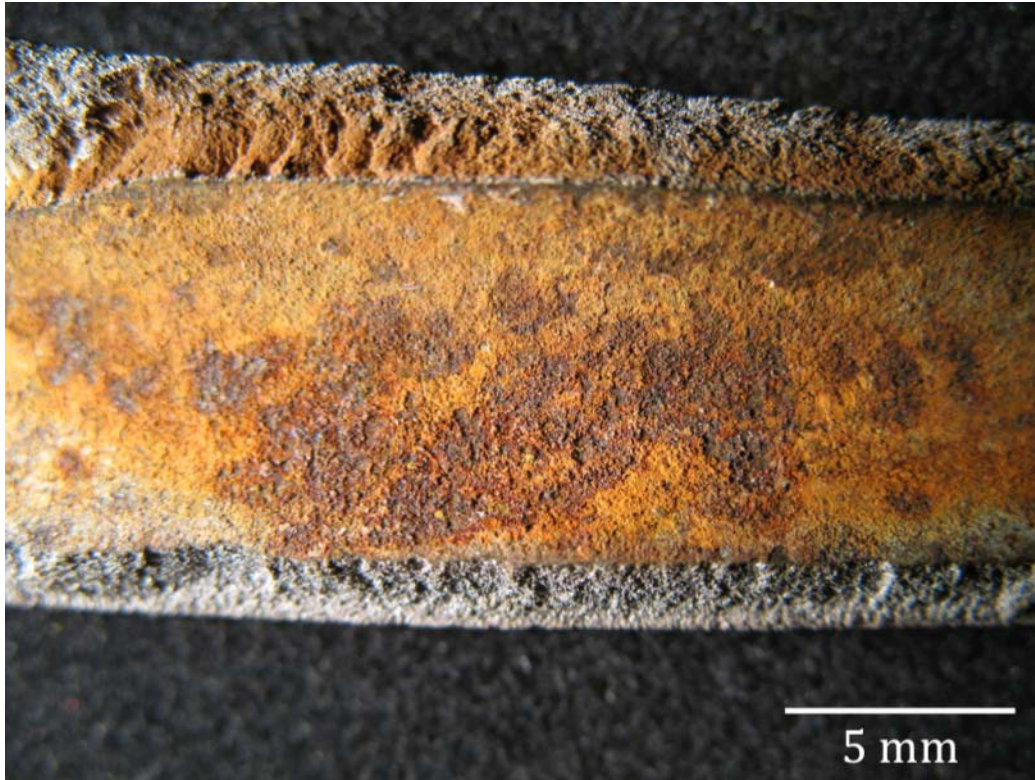
FIGURE 3 High Magnification Picture of Fracture Surface of #6YC Sliver as shown in Figure 1.
