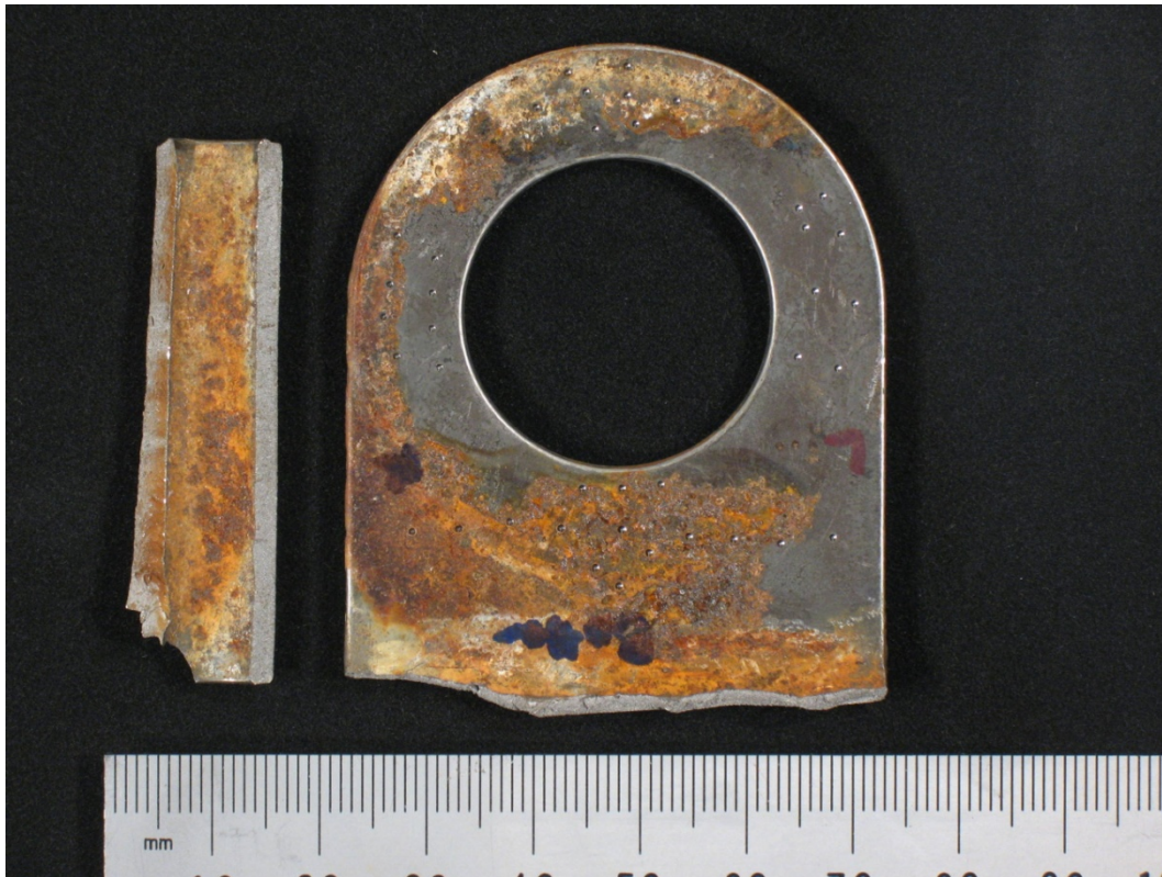
FIGURE 1 Photograph of Corroded and Failed Yoke Sample #6YC.
