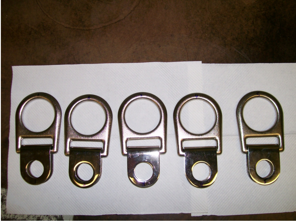
FIGURE 5 Five As-Received Ni-5% P Coated Yoke/D-ring Assemblies.
