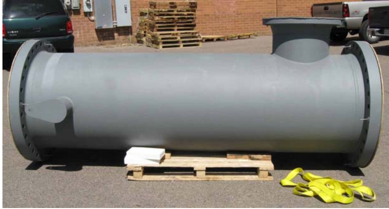
Figure 5 Thermal Oxidizer Shell
