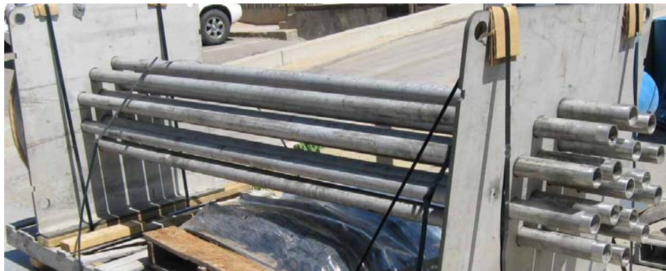
Figure 4 Thermal Oxidizer Core Tubes
