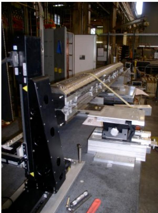
End on view of Undulator with Steel Beampipe.
