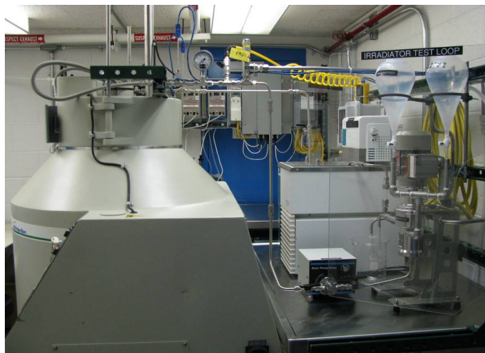
Figure 2. View of radiolysis/hydrolysis test loop showing gamma irradiator (center foreground), centrifugal contactor (right), recirculation pump (center), and temperature-controlled water bath (center back).
