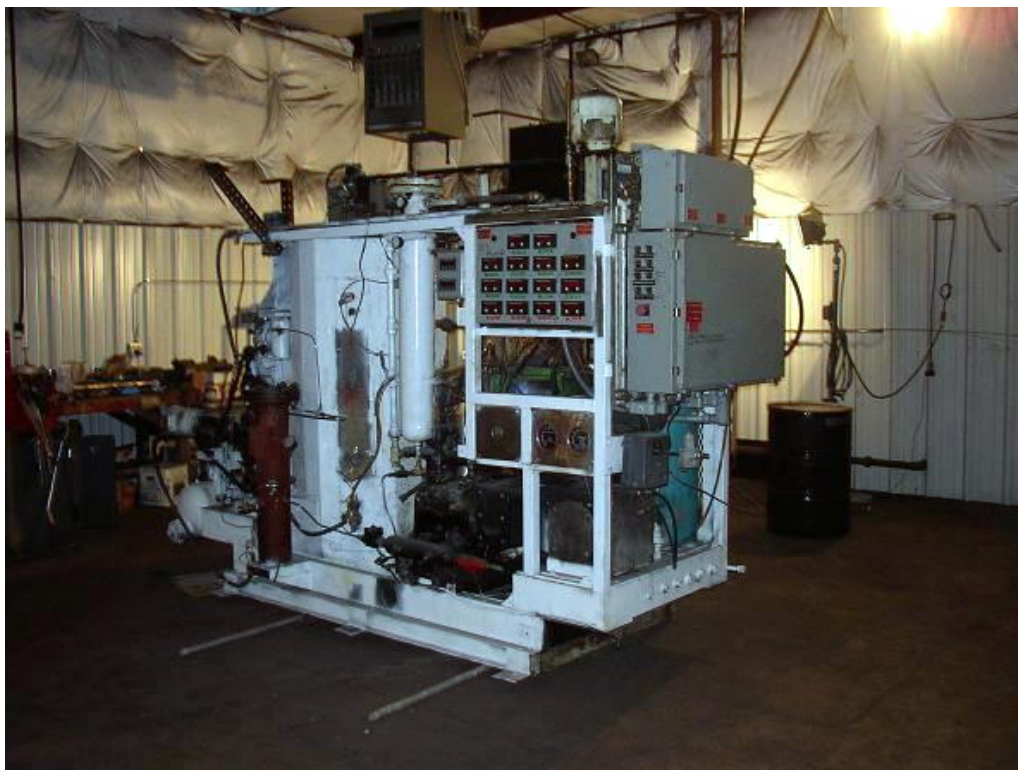
Figure 3. BCT Prototype gasifier installed at WRI
