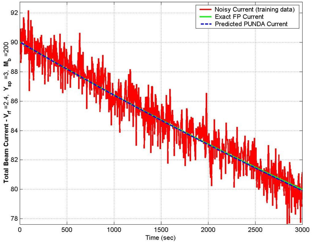
**Figure 6:** Prediction of electron beam decay using PUNDA model where gap voltage ( $V_{rf}$ ) is reduced from 3.2 in Fig. 5 to 2.4, resulting in a larger loss in beam current.
