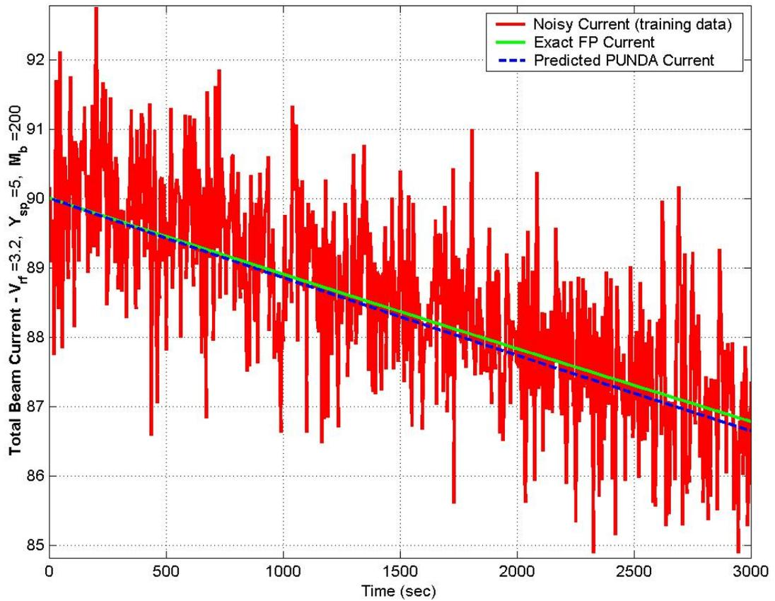
**Figure 5:** Prediction of electron beam decay using PUNDA model where gap voltage ( $V_{\text{rf}}$ ) and vertical scraper position ( $Y_{\text{s}}$ ) are the same as in Fig. 2, while number of bunches ( $M_{\text{b}}$ ) is reduced 200. The beam displays a linear decay (from a lower value of initial current compared to that in Fig. 2).
