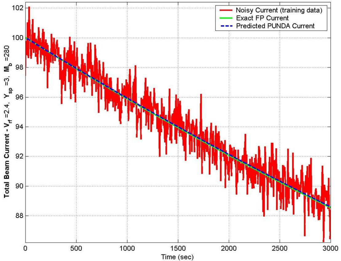
**Figure 3:** Prediction of electron beam decay using PUNDA model where gap voltage ( $V_{\text{rf}}$ ) is reduced from 3.2 in Fig. 2 to 2.4, resulting in a larger loss in beam current.
