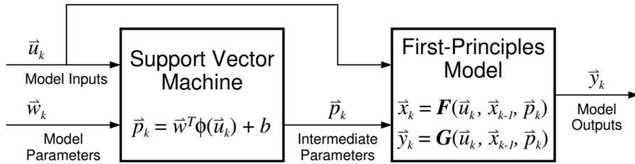
**Fig. 1:** Block Diagram of the Combined SVM and FP blocks that will be used to model nonlinear beam matrix and estimate the onset of a fault.
