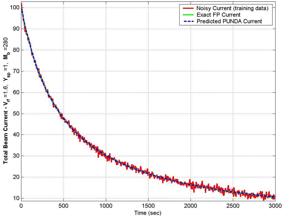
**Figure 4:** Prediction of electron beam decay using PUNDA model where gap voltage ( $V_{\text{rf}}$ ) is reduced to 1.6 and vertical scraper position ( $Y_{\text{s}}$ ) is set to 1. The beam decay in this case demonstrates an exponential decay (to significantly lower values of beam current) over the hour long simulation horizon.
