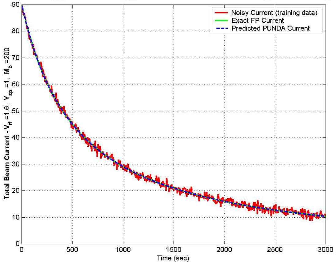
**Figure 7:** Prediction of electron beam decay using PUNDA model where gap voltage ( $V_{\text{rf}}$ ) is reduced to 1.6 and vertical scraper position ( $Y_s$ ) is set to 1, while number of bunches ( $M_b$ ) is kept at the level of Fig. 5. The beam decay in this case demonstrates an exponential decay (to significantly lower values of beam current) over the hour long simulation horizon.
