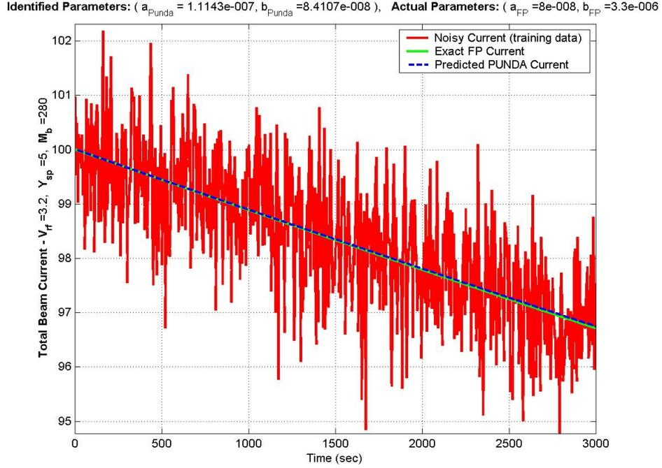
**Figure 2:** Prediction of electron beam decay using PUNDA model. The beam decay is accurately predicted while acceptable estimates of the decay model parameters are obtained. The actual parameter values used in the FP model of Eq. (25) are reflected in the title of the plot. Under the given beam operating conditions, indicated along the y axis, beam current decays *linearly* over the course of approximately one hour of operation.
