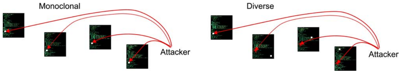
Figure 2.2. Identical versus diverse implementations. Turing completeness and undecidability cause security holes to be unknowable in the general case to programmers, users, and attackers. Implementations that are identical (monoclonal) are equally susceptible to the discovery of a security hole by an adversary. Diverse implementations are less so, depending on the number of variants.
