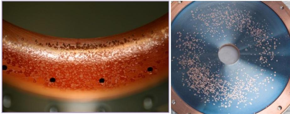
Figure 12. Damaged iris surface and Cu deposition on the Be window.
