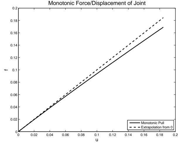
Figure 4.27. The force history of the joint resulting from a very low amplitude ( A_0 = 0.005 ) base excitation corresponds to the above portion of the monotonic force-displacement curve for the joint. Also shown is the tangent stiffness at zero load.
