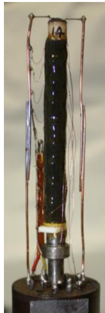
Figure F4. Propellant strand prior to burn. Strand is encapsulated in Halthane 88-2 in order to prevent flame flashing down the side of the strand and to hold assembly together. Burn wires are soldered to a base that is connected to an oscilloscope. A wire is embedded in the cardboard tube containing the BKNO 3 and HNS pellet and is used to ignite the materials.
