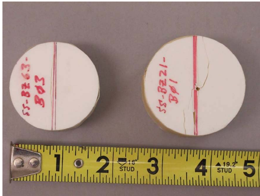
Figure 3 Post-test images of samples SS-BZ63-B03 and SS-BZ21-B01. Note vertical diametric crack; this is the crack along which these samples broke when deformed.
