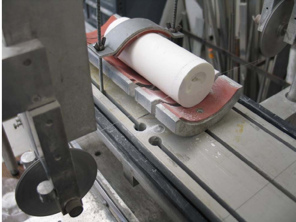
Figure 2 Example of salt core being cut to length using a wire saw.
