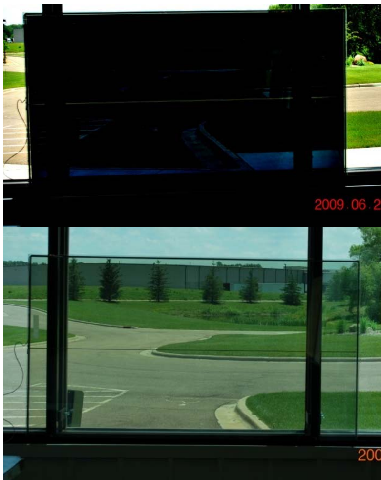
Figure 19 – Photographs of a large area device (60"x34") produced using the techniques described in this report, shown in both the clear and colored states.
