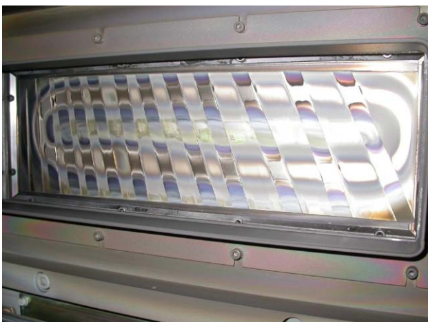
Figure 4 – Photograph showing the method of producing a composite target by clamping strips of one material to a target of another.
