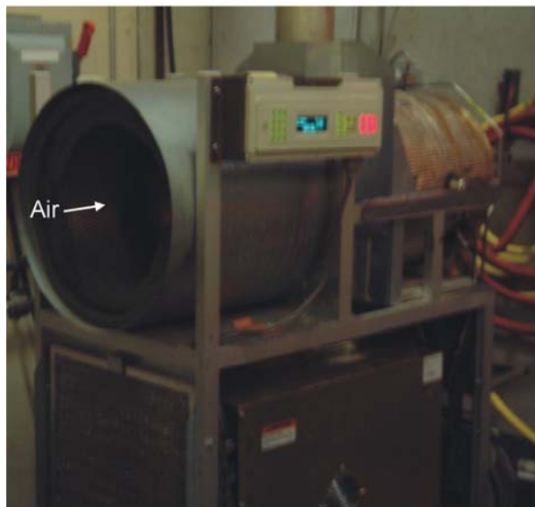
Figure 2. C30 microturbine utilized for low-Btu testing (3).
