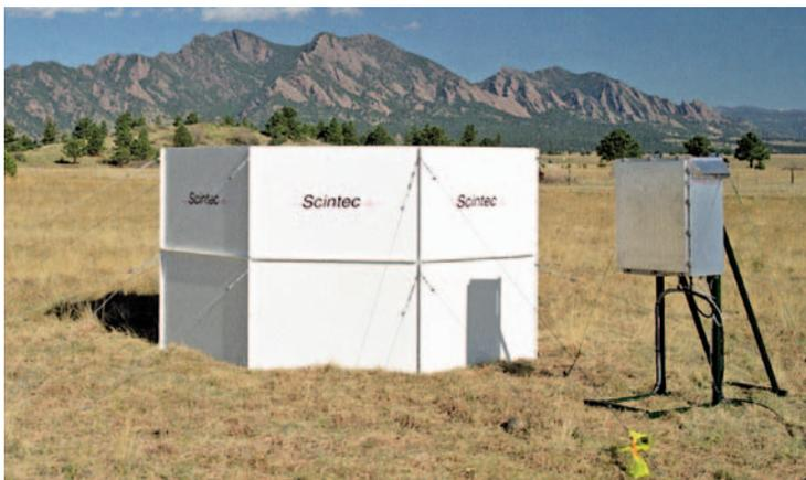
Shown here is a close-up of sonic detection and ranging (SODAR) system enclosure and associated electronics equipment at the NWTC.
