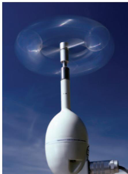
The cup anemometer shown here provides accurate measurements of wind speed.
