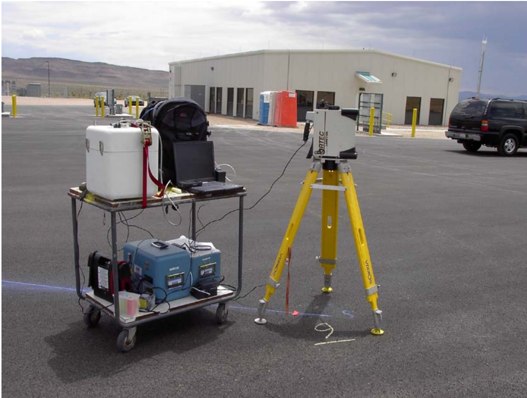
Figure 1: Setup for performing the static measurements. The HPIC and VECTOR are on top of the cart while the HPGe is on the tripod. Batteries on the bottom of the cart were used to power the various systems throughout the day.
