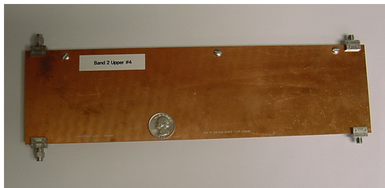
Figure 12. Picture of the FIR filter depicted by the schematic of Fig. 11. This board is about 17" long and has a delay of around 3.1 nsec.
