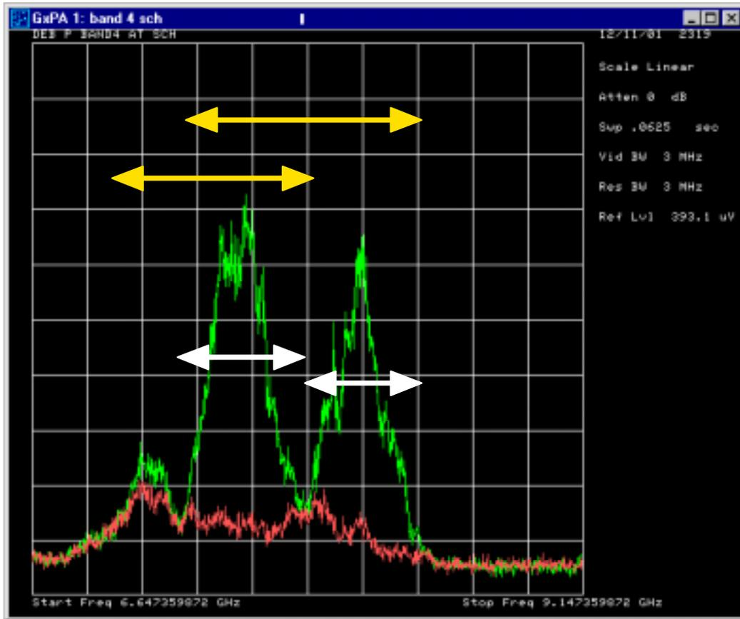
Debuncher Band 4 Momentum Signal to noise.
