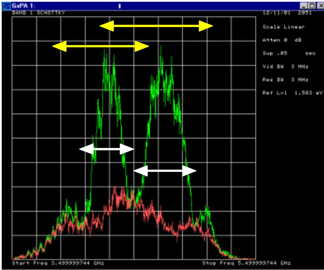
Debuncher Band 1 Momentum Signal to noise.
