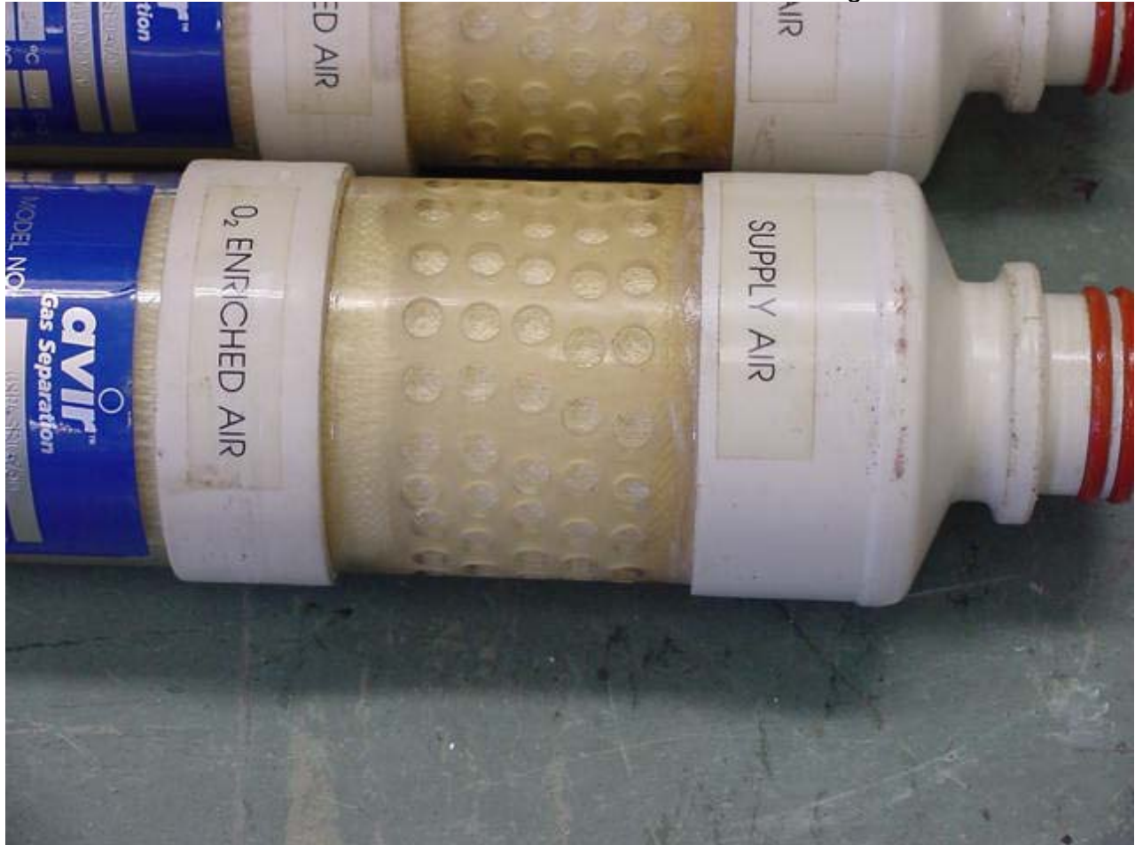
Figure 19: Permeate Vent Crossbores
