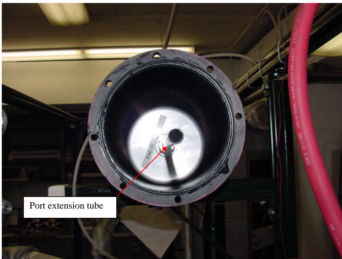
Figure 30: Module in place prior to installation of an end cap
