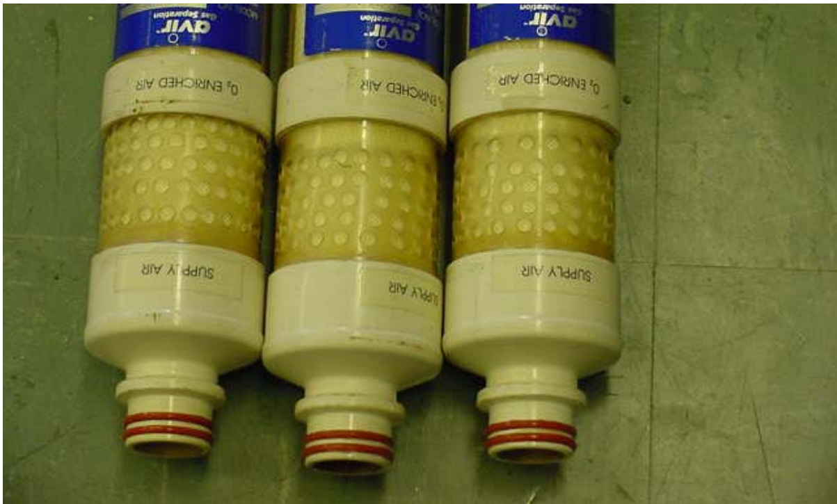
Figure 20: Dual O-rings on Module Elements
