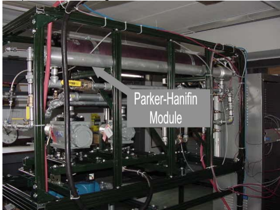
Figure 33: Membrane test bench with Parker-Hanifin module
