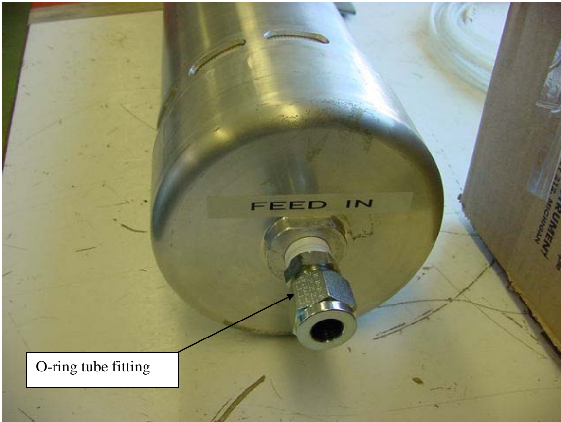
Figure 28: Prism Alpha 5 module fitted with 1/2 inch tubing fitting.
