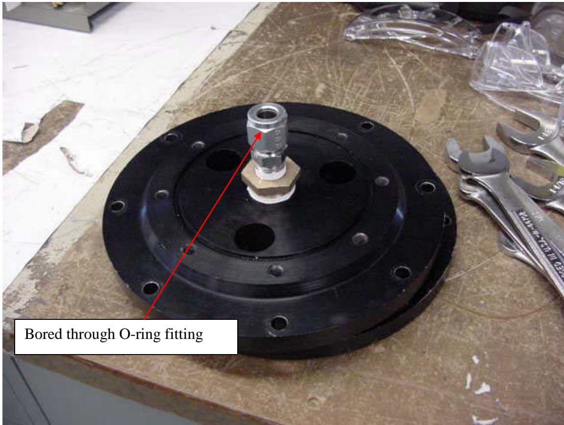
Figure 29: End flange with bored through o-ring fitting
