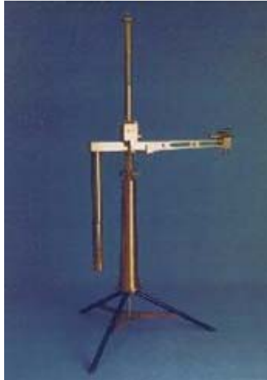
Figure 13. Early torsion balance Gradiometer developed by Baron Roland von Eotvos in 1890.
