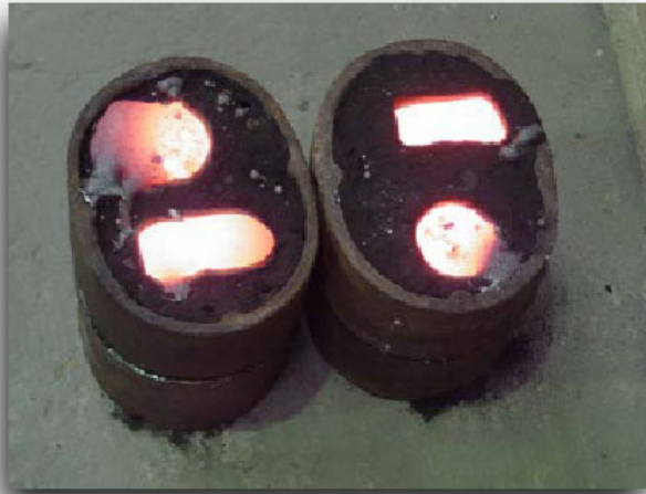
Iron castings in sand molds with fly ash cores.
