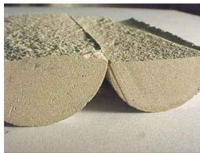
Figure 2: Different failure modes of Class C samples after testing. (Without fiber [left] and with 1.0 % fiber [right])
