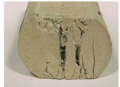
Figure 2: Different failure modes of Class C samples after testing. (Without fiber [left] and with 1.0 % fiber [right])
