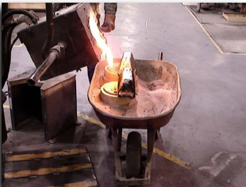
Pouring gray iron into sand molds with cores made of fly ash.
