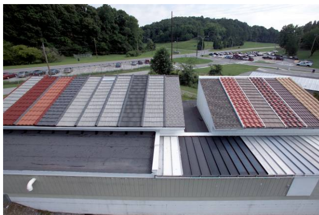
Fig. 3. Two south-facing assemblies of steep-slope attics were placed atop ESRA, and stone-coated metal shakes, S-mission tile, and painted metal shakes were installed by MCA.
