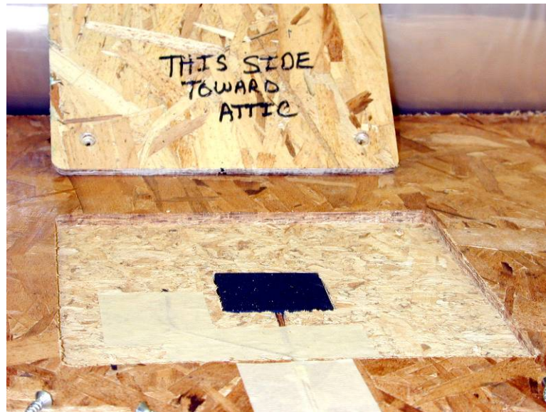
Fig. 6. Heat flux transducer embedded in the roof deck to measure heat flow penetrating stone-coated metal shake and attic.
