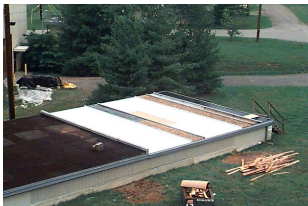
Fig. 2. The envelope systems research apparatus (ESRA) is a one-story building for testing low- and steep-slope roof products.
