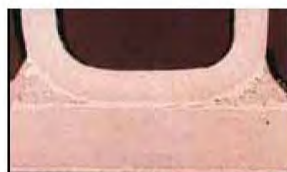
Typical PFHE brazed joint
