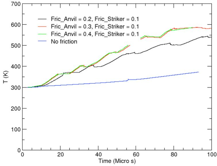
Figure 4. Temperature profile inside HE\_1 sample at  $t = 80ms$  after impact (obtained from ALE3D simulation).
