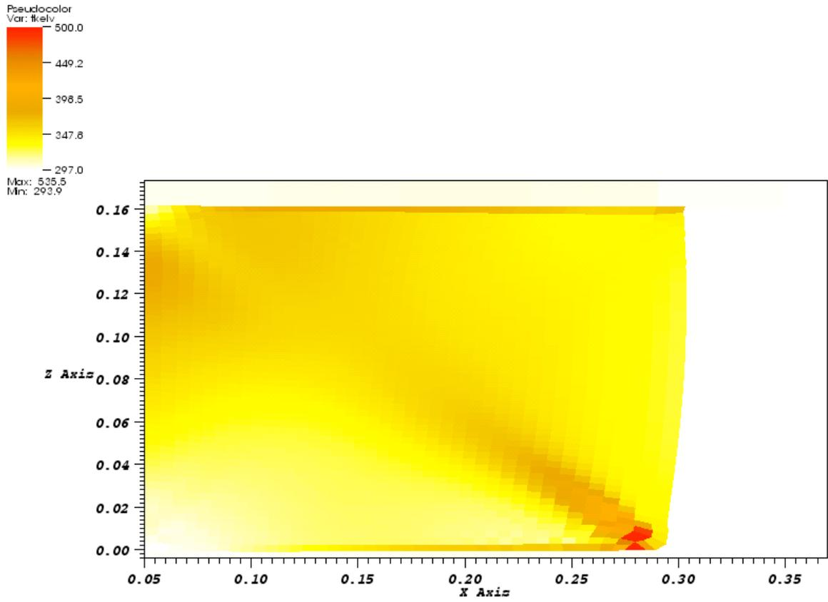
Figure 5. Pressure profile of JA2 obtained from a five-center inside burn model.
