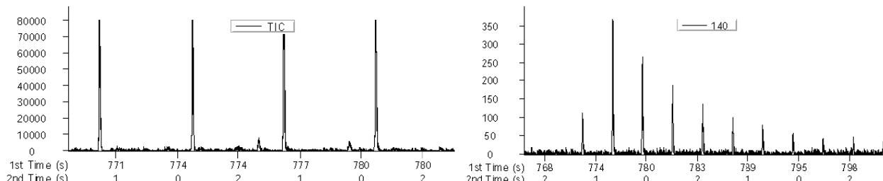
EI chromatograms supporting identification; TIC on left; EIC ( $m/z$  140) on right
