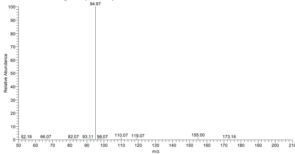
LC/MS/MS spectra – product spectra of parent  $[M-H]^-$  m/z 137. Top: Urine sample S6. Bottom: reference standard of **Isopropyl methylphosphonate**
