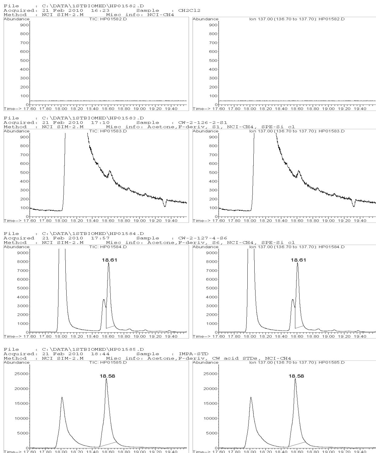
CI chromatograms supporting identification; TIC on left; EIC ( $m/z$  137) on right.
