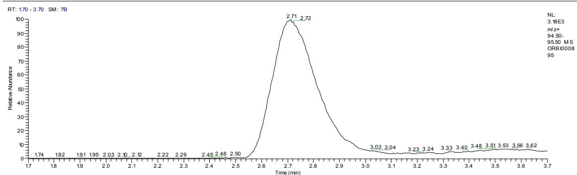
LC/MS/MS EIC (m/z 95) chromatograms. Top: water blank. Next: Urine blank S1. Third: Urine sample S3. Bottom: reference standard of **Isopropyl methylphosphonate**
