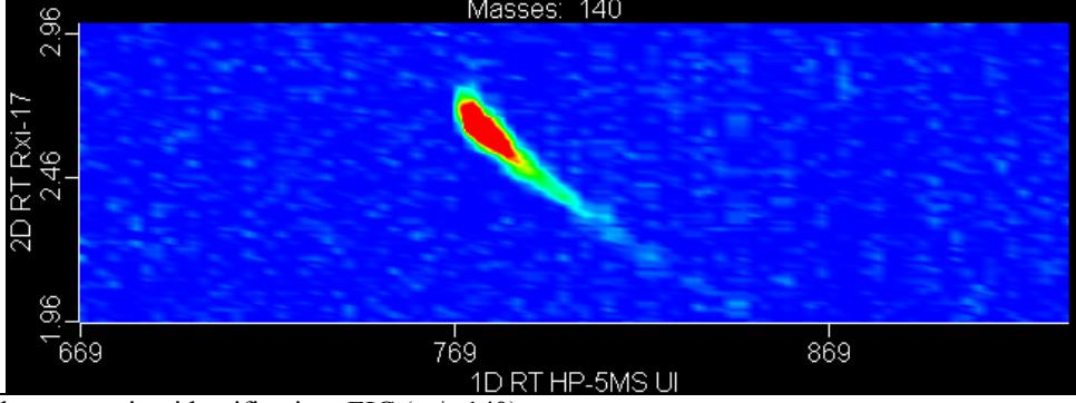
2D Contour plot supporting identification; EIC (m/z 140)
