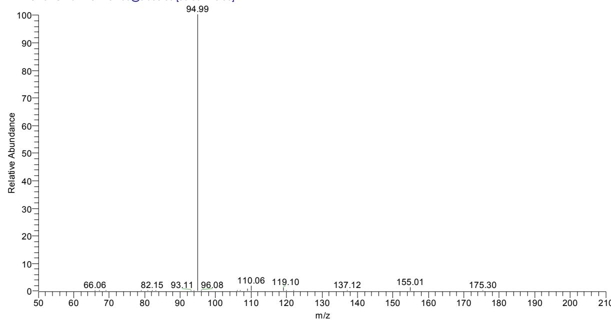
LC/MS/MS spectra – product spectra of parent  $[M-H]^-$  m/z 137. Top: Urine sample S3. Bottom: reference standard of **Isopropyl methylphosphonate**
