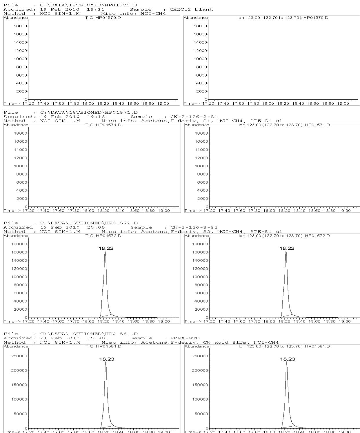
CI chromatograms supporting identification; TIC on left; EIC ( $m/z$  123) on right.
