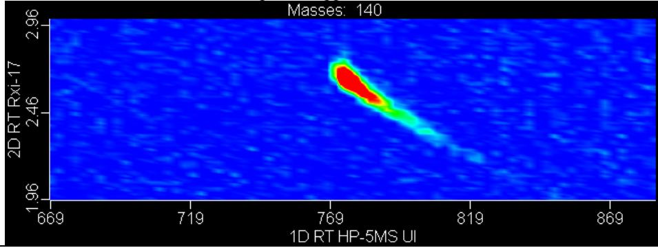
2D Contour plot supporting identification; EIC (m/z 140)
