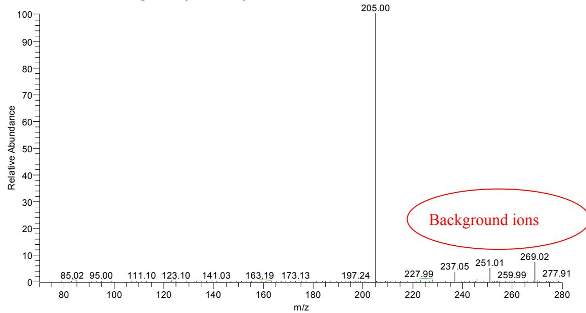
LC/MS/MS spectra – product spectra of parent  $[M+Na]^+$  m/z 269. Top: Urine sample S5. Bottom: reference standard of 1,1'-Sulfonylbis[2-(methylsulfinyl)ethane].
