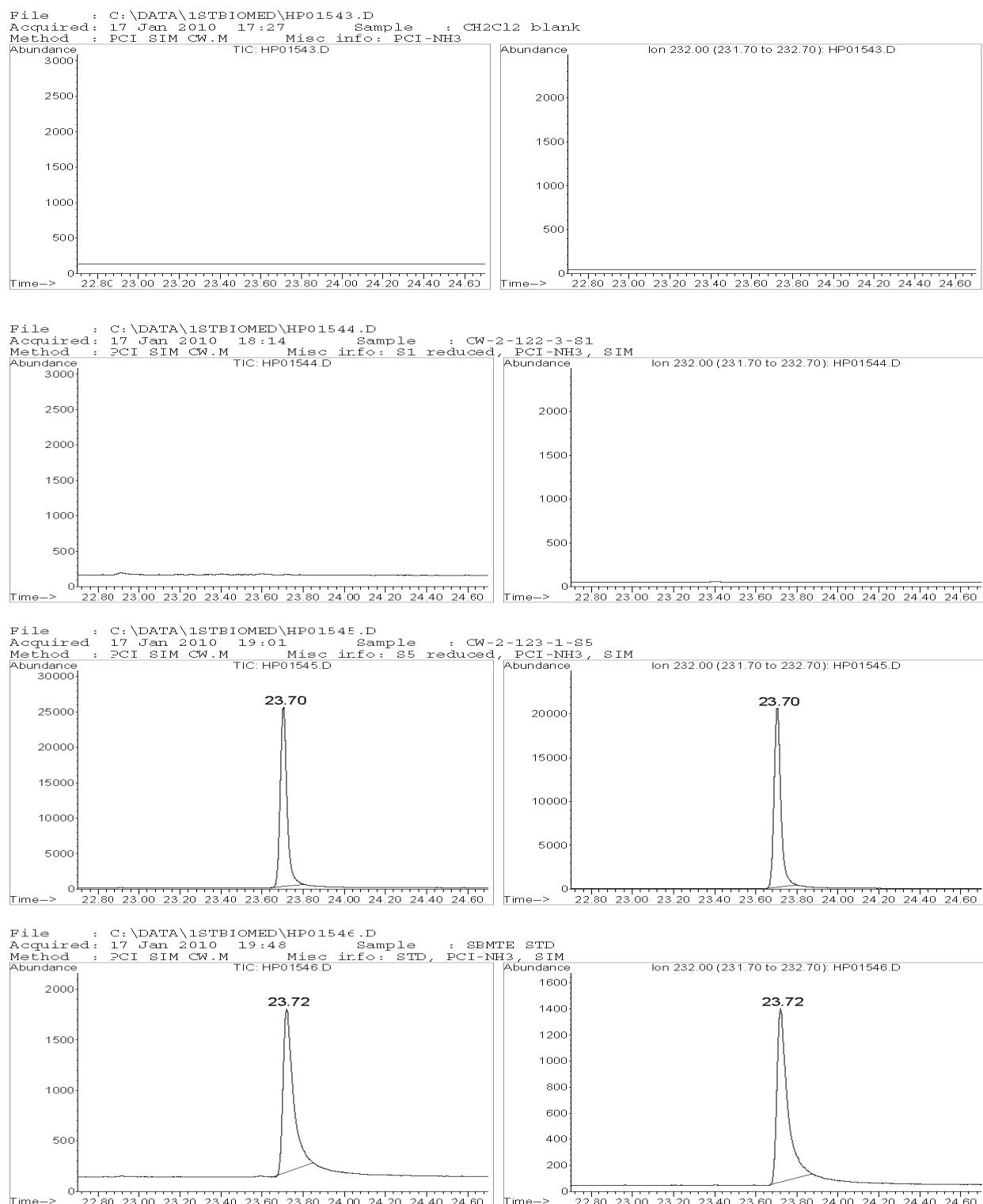
CI chromatograms supporting identification; TIC on left; EIC ( $m/z$  232) on right.
