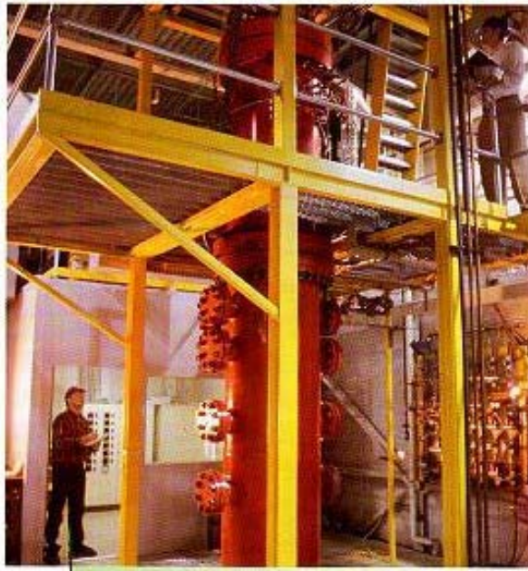
Figure A1. IPST's Pressurized Entrained Flow Reactor
