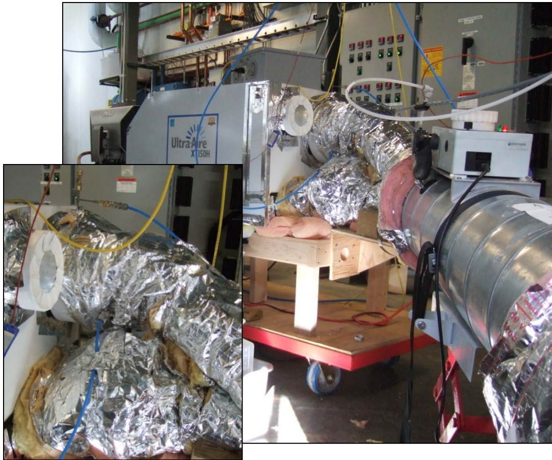
Figure 6. Photograph of Ultra-Aire XT150H test setup
