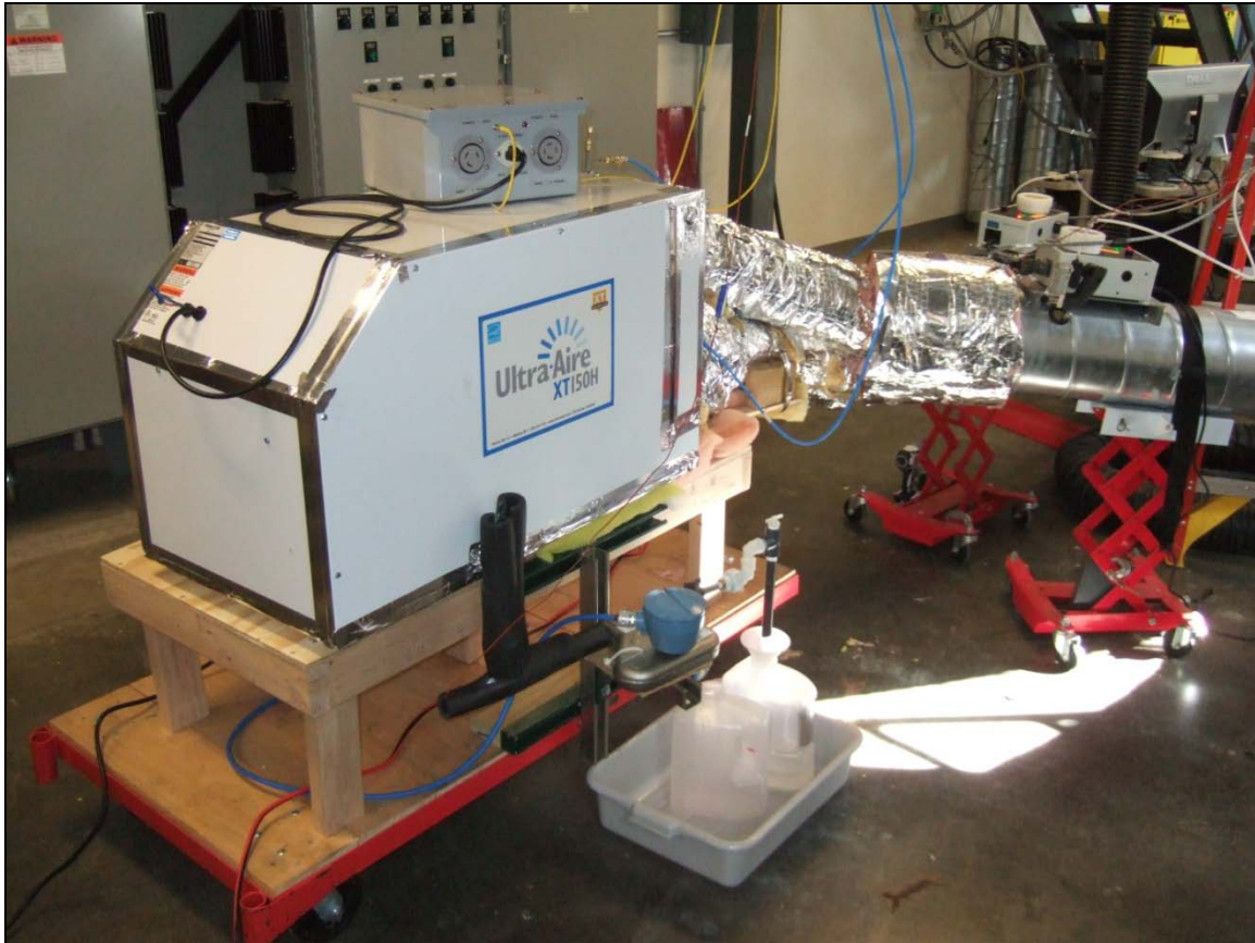
Figure 5. Photograph of Ultra-Aire XT150H test setup
