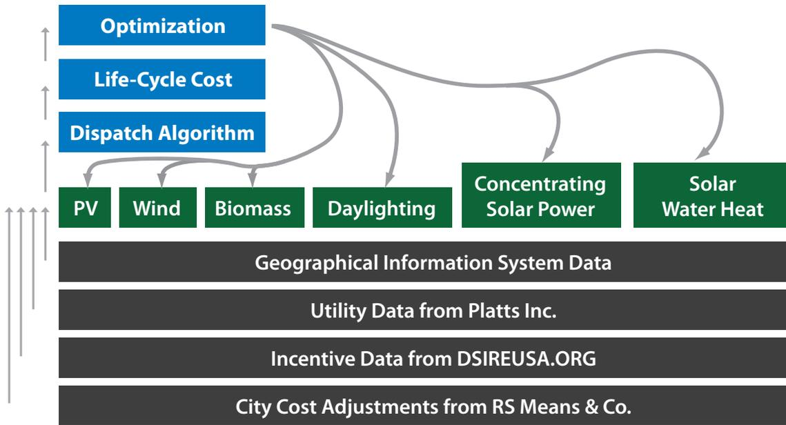
*The REO tool analyzes a variety of data used to identify the optimal combination of renewable energy technologies needed to minimize the life-cycle cost of achieving the net-zero goal.*
