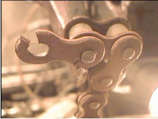
Figure 1. Photographs of damaged bridge drive chain links.
